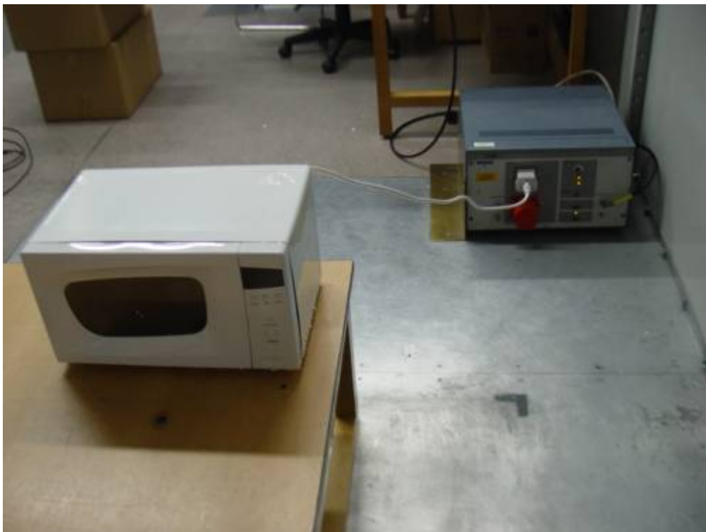
Photo 2 Conducted Disturbance Test (WP700D-N20)
