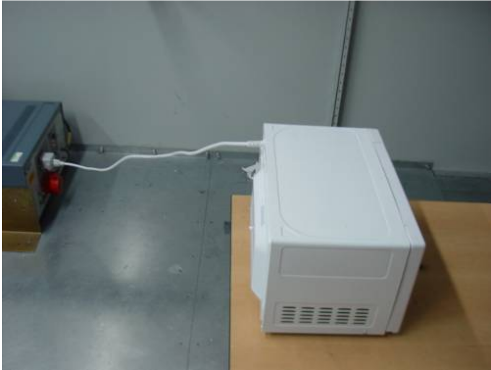
Photo 2 Conducted Disturbance Test (WP700D-N20)
