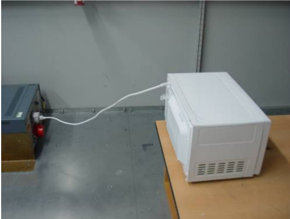
Photo 4 Conducted Disturbance Test (WP700D-S20)
