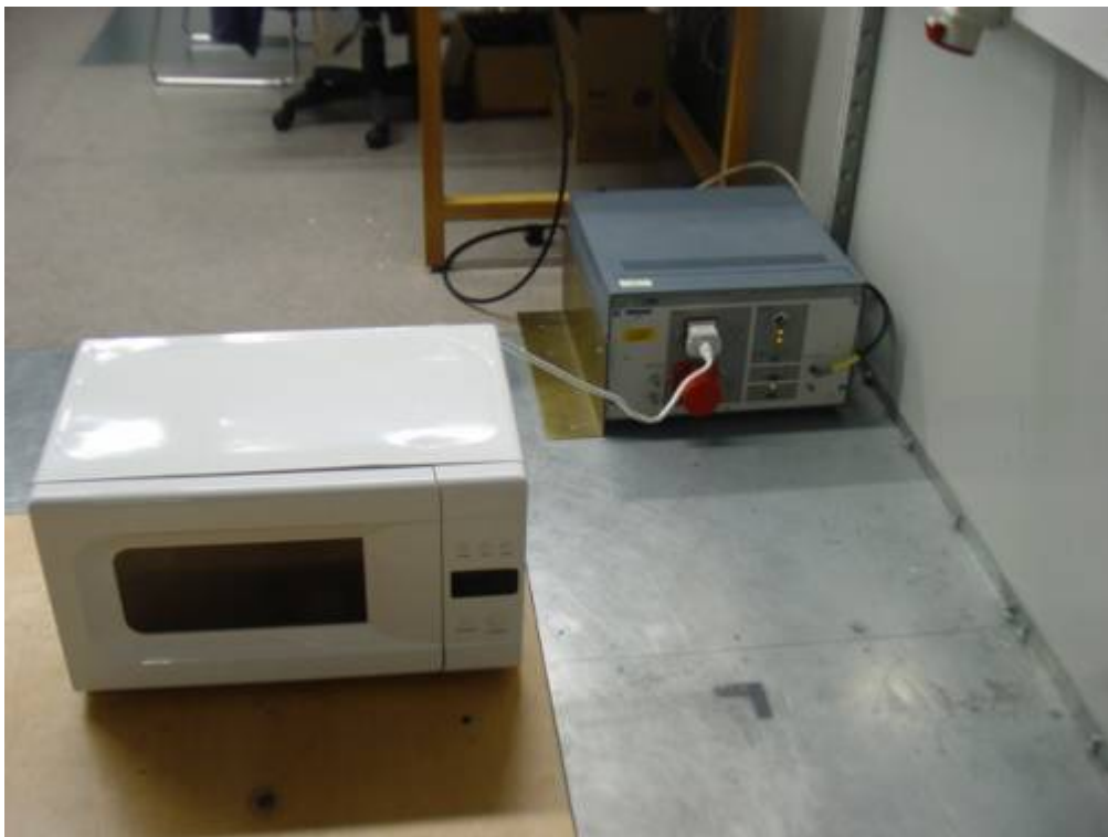
Photo 4 Conducted Disturbance Test (WP700D-S20)
