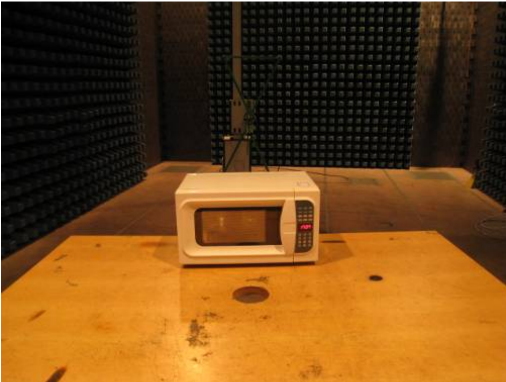
Photo 20 Radiated Disturbance Test (above 1GHz) (MEW50M-A)
