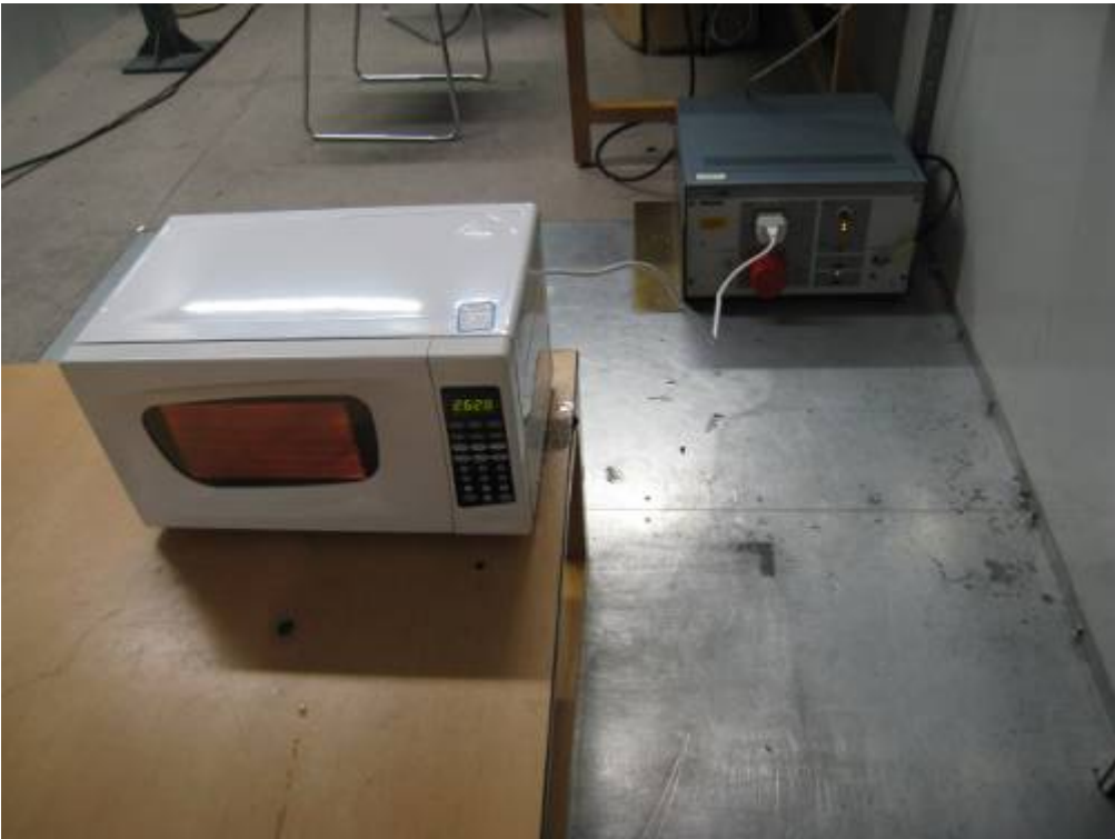
Photo 2 Conducted Disturbance Test (MEW50N-A)
