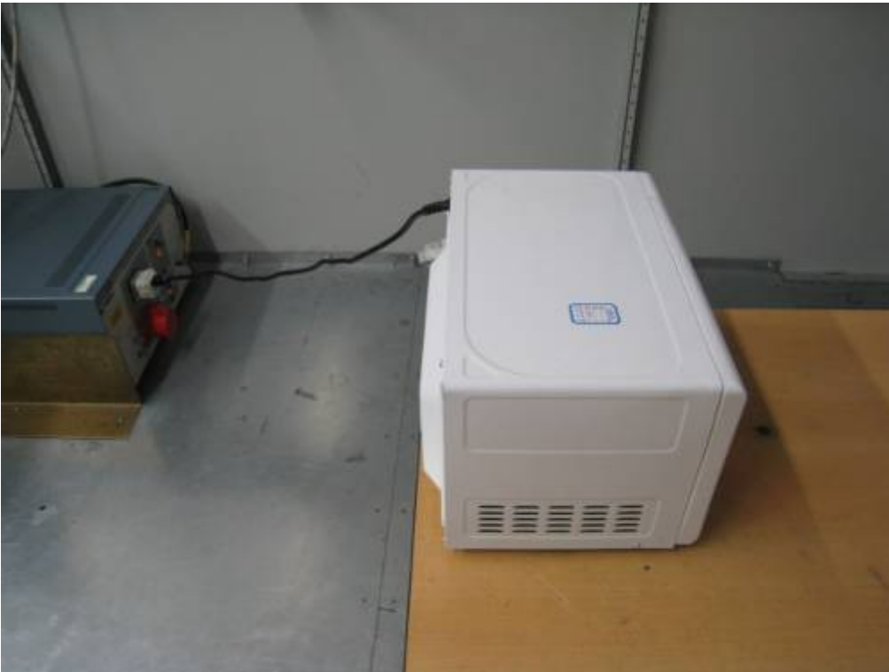
Photo 6 Conducted Disturbance Test (MEW50B-A)
