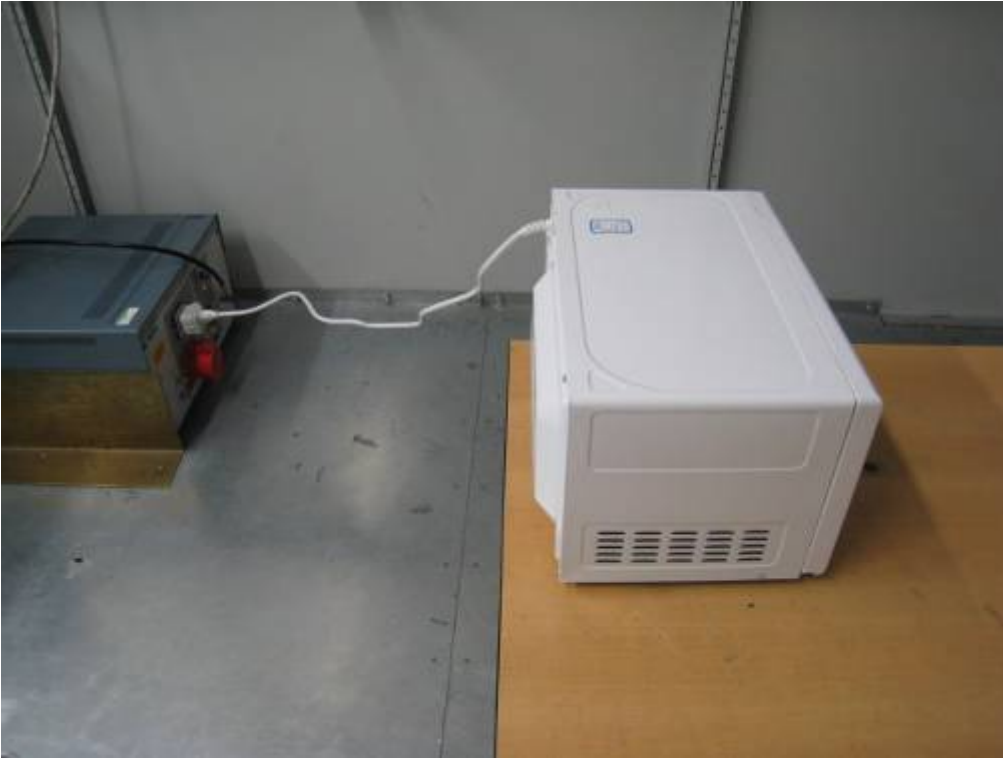
Photo 4 Conducted Disturbance Test (MEW50S-A)
