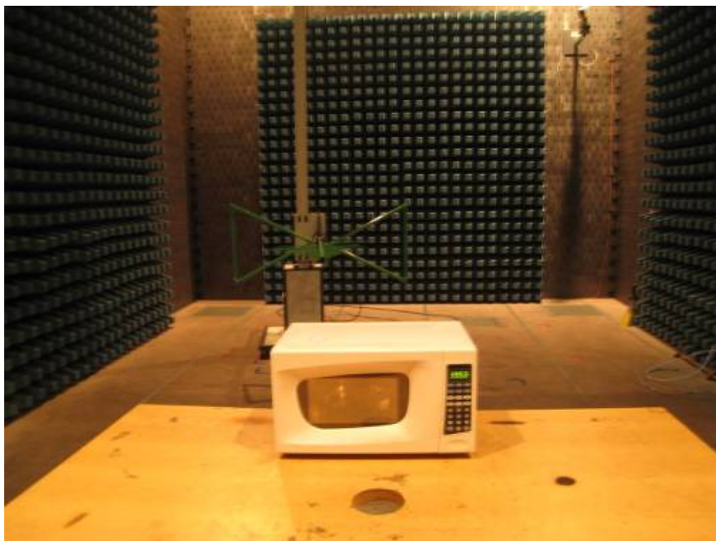
Photo 12 Radiated Disturbance Test (above 1GHz) (MEW50N-A)
