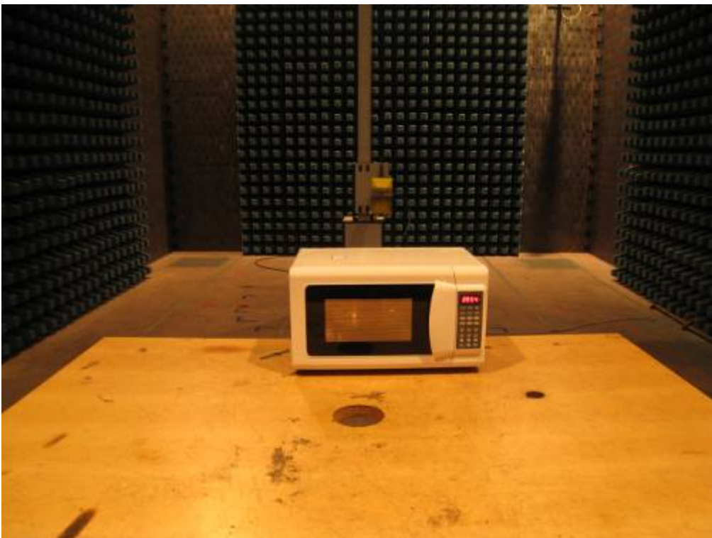
Photo 16 Radiated Disturbance Test (above 1GHz) (MEW50B-A)
