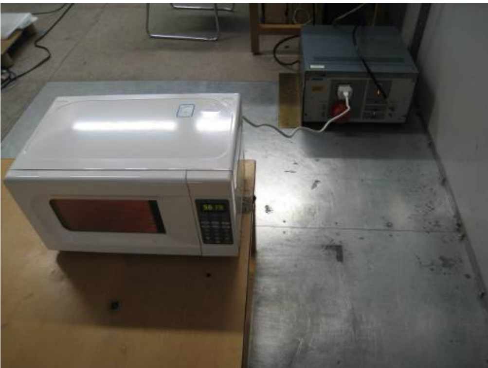
Photo 4 Conducted Disturbance Test (MEW50S-A)
