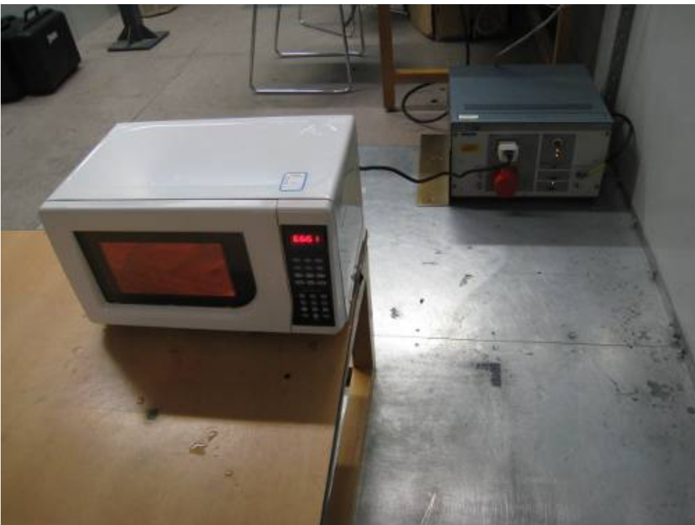
Photo 8 Conducted Disturbance Test (MEW50D-A)
