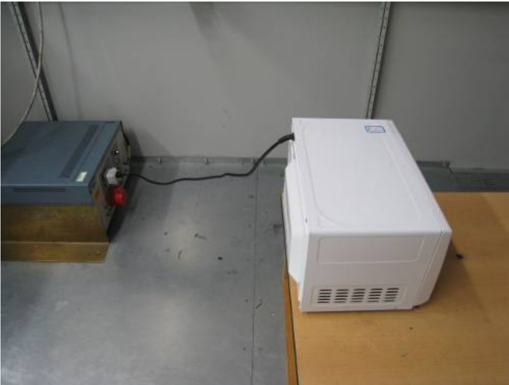
Photo 8 Conducted Disturbance Test (MEW50D-A)
