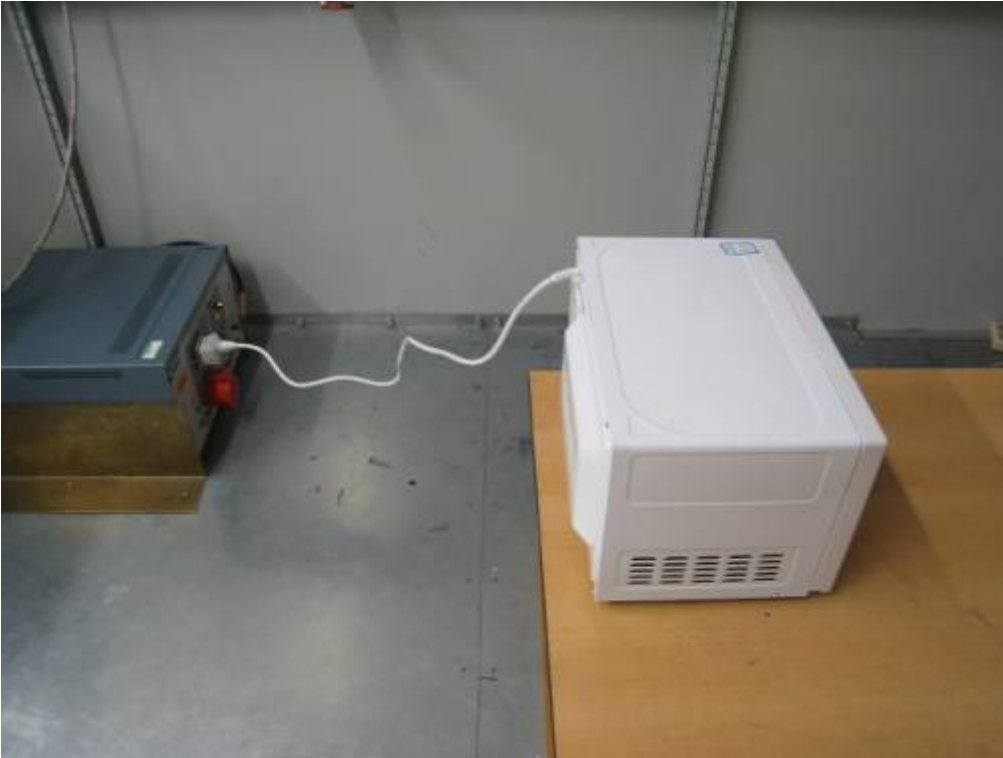
Photo 2 Conducted Disturbance Test (MEW50N-A)
