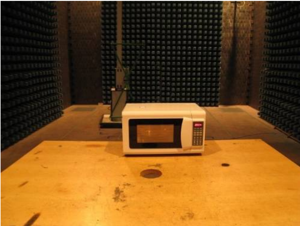
Photo 16 Radiated Disturbance Test (above 1GHz) (MEW50B-A)
