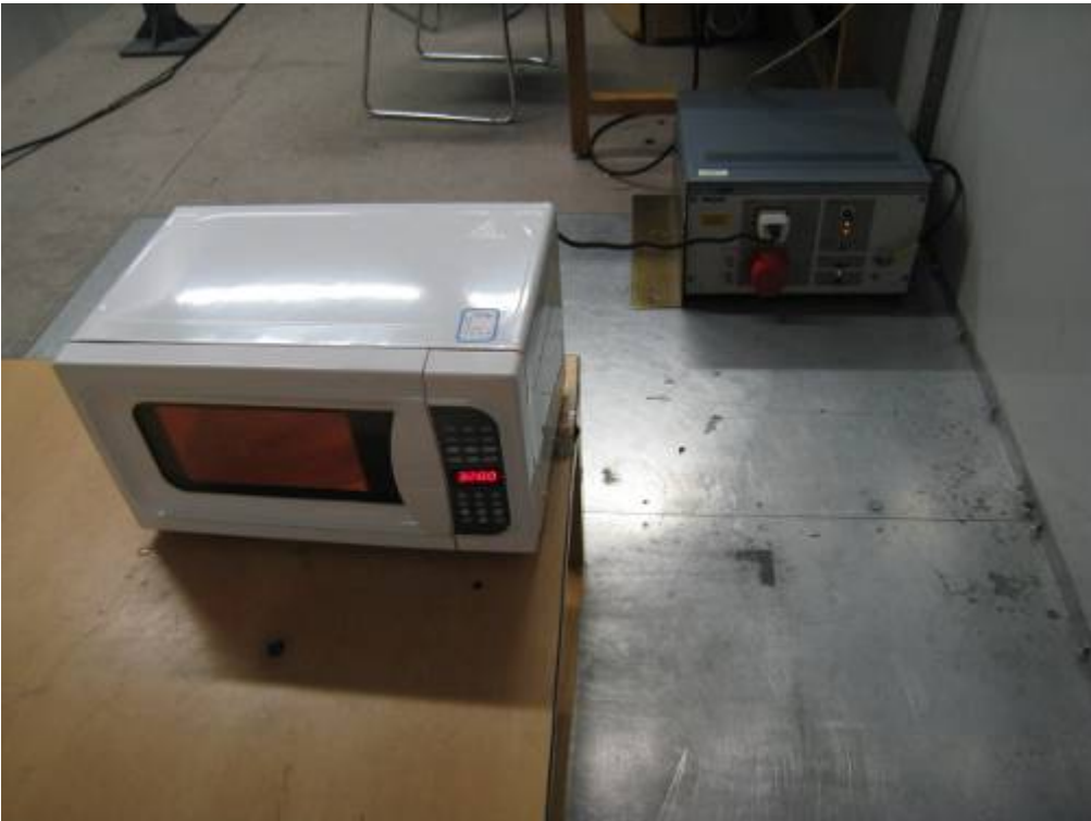
Photo 10 Conducted Disturbance Test (MEW50M-A)
