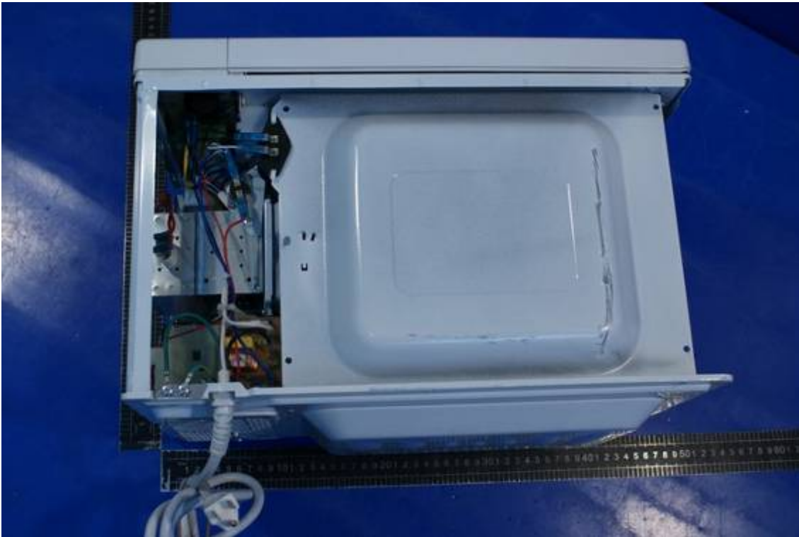
Photo 1 Internal photo of EUT (MEW50N-A)
