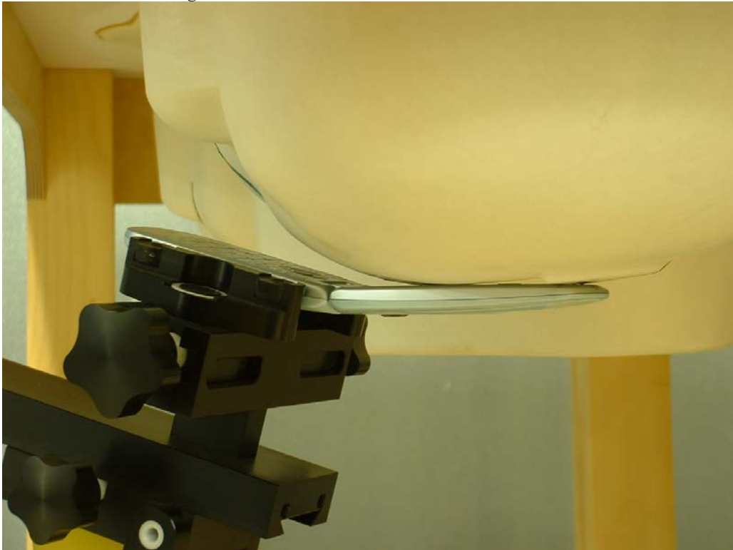
Configuration 1 (Left Head – Cheek/Touch Position)
