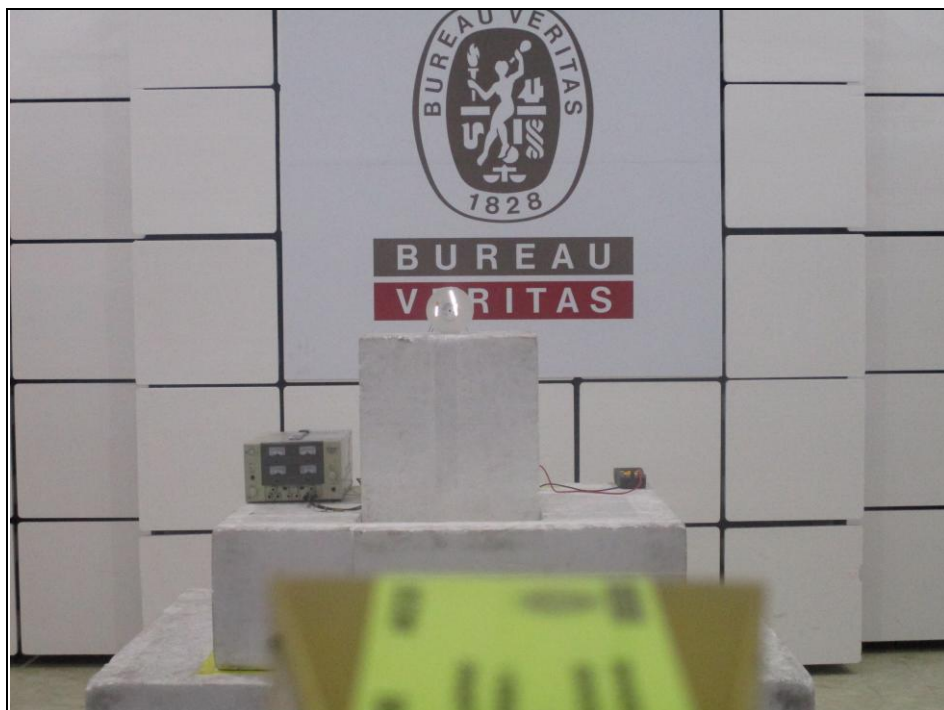
Radiated Emission Test (50GHz ~ 55GHz)
