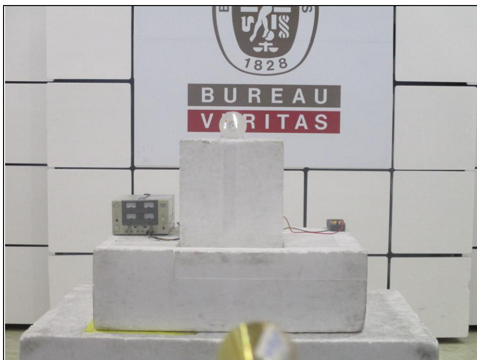
Radiated Emission Test (50GHz ~ 55GHz)
