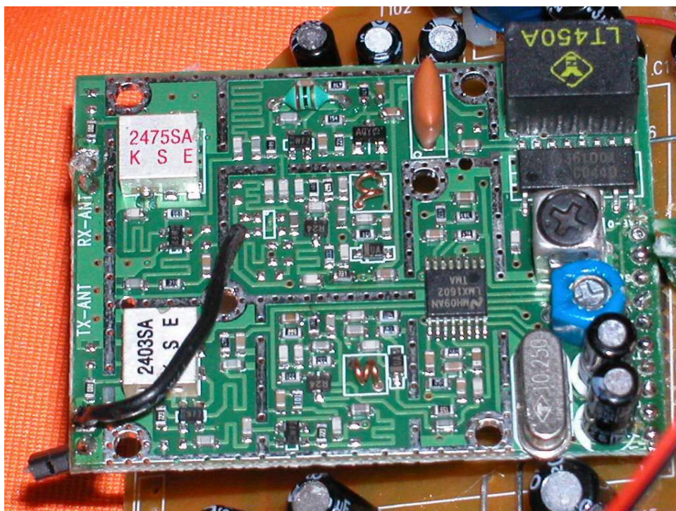
Base Oscillator PCB comp side
