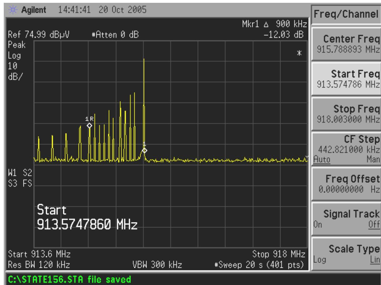
At the marker 1R, we switched off the transmission of the equipment under test.
