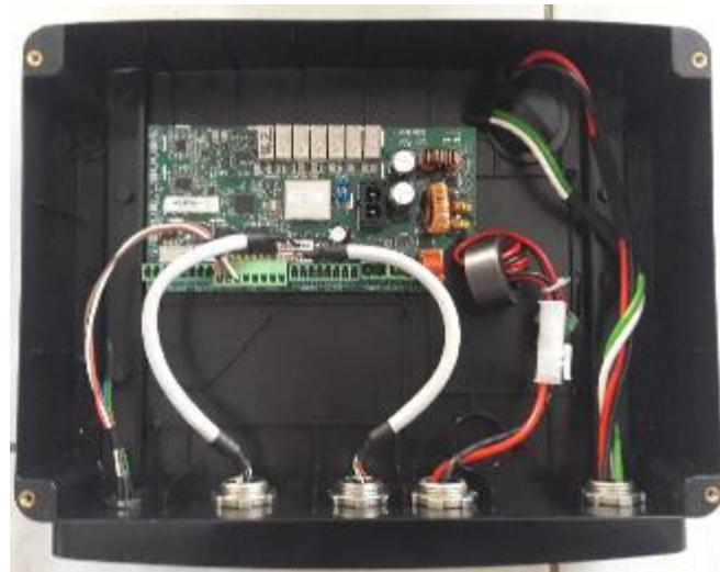
The RM5 is a standalone near field 12VDC RFID reader, design to read ISO11784/5 compliant passive tags. The module consists of an ARM based microcontroller clocked by 17.1776MHz VCXO. An internal PLL generates a 60MHz internal clock that is not used outside the CPU core.
