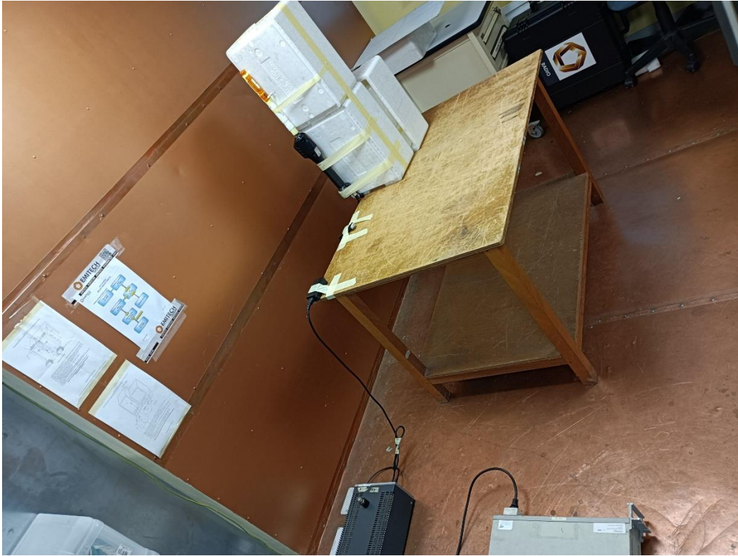
AC Conducted Setup with 50 ohms load
