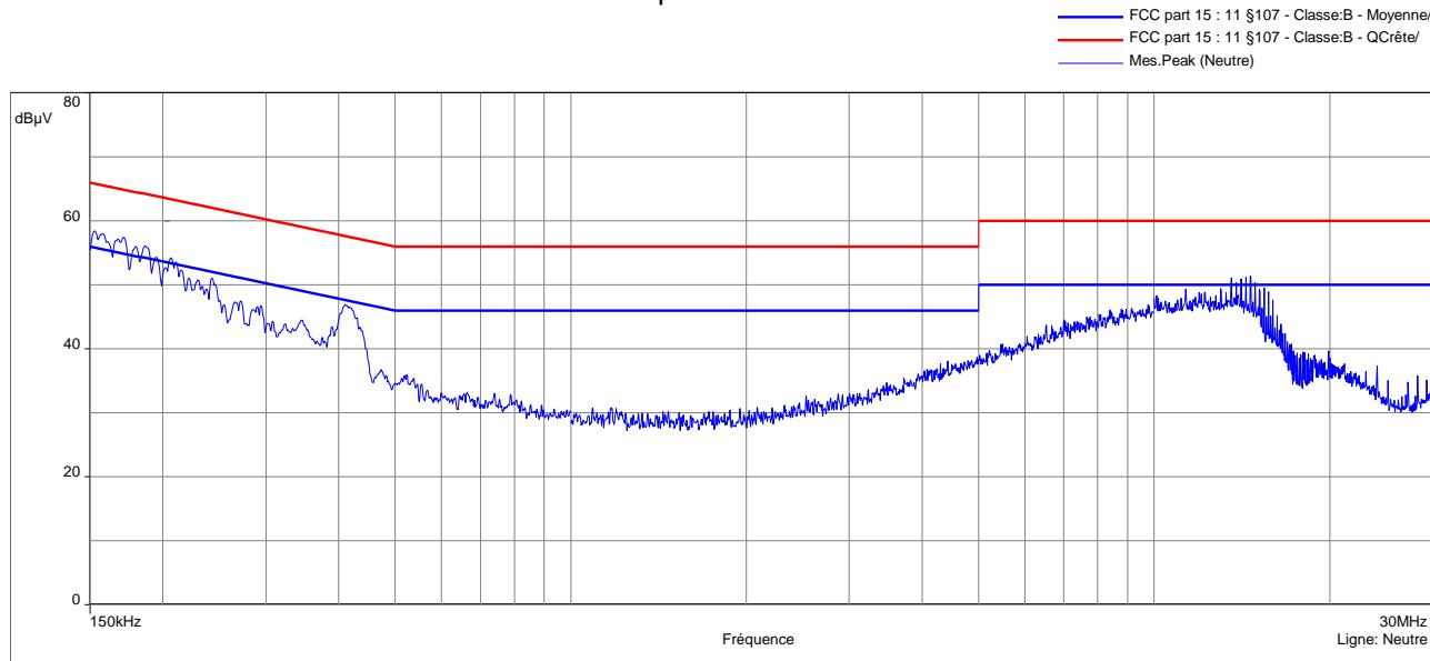
Curve N° 2: measurement on the Line with peak detector
