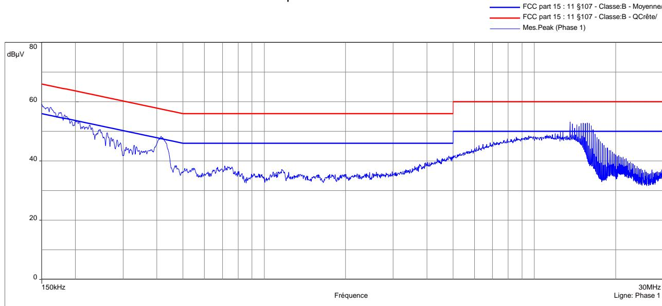
The frequencies which are not 6 dB under the Quasi-peak limit are then analyzed with Quasi-peak detector.
