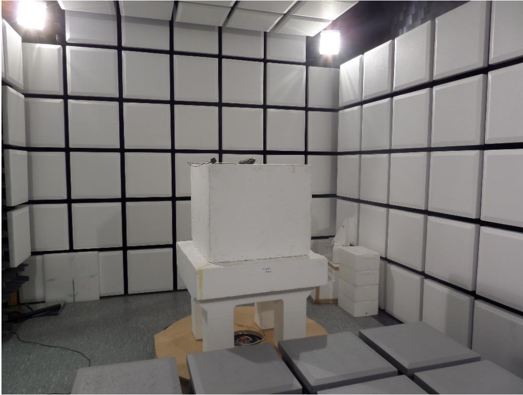
Anechoic room – Position 2 supplied by AC/DC Adapter
