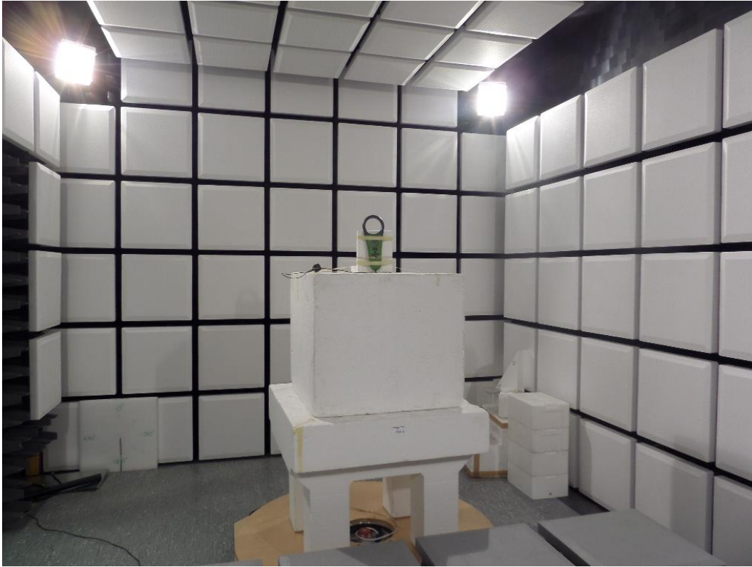
Anechoic room – Position 1 supplied by AC/DC Adapter
