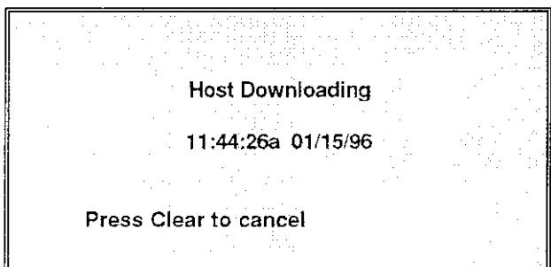
Note: If the host initiates the download/upload process, then this screen will automatically appear. However, this will not be allowed if the TCP-CO is in the program mode or currently in the loading sequence. Once all the new shift information has been received, the following will be displayed:
