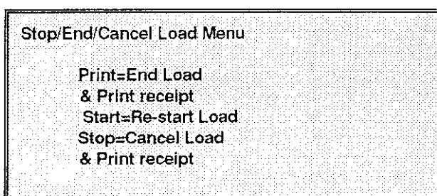
This menu will also be displayed for permissive, zero flow or volume cutoff options. If cancel load is selected, the stop record will be flagged as aborted and cannot be re-selected for another load. If it is desired to load this stop again, use the add load menu to copy this stop and create a new stop. Then proceed as before.
