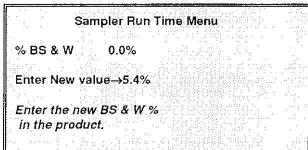
Enter the new percentage of sediment and water. Pressing 'ENTER' will store the new percentage and the TCP will recalculate the Dry Product Volume using the new entries and return the unit to the Sampler Run Time Menu.
