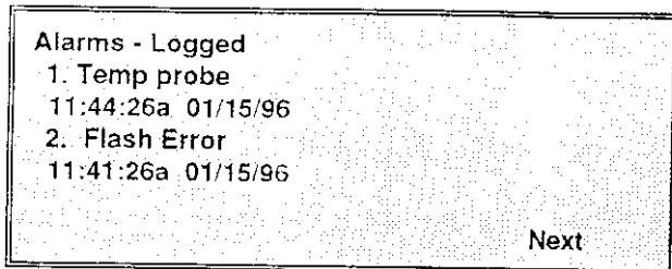
The TCP will log six pages of alarms with three alarms on a page. When all six pages are full the next alarm that occurs will be displayed and the first one that had occurred will be replaced. Pressing the up and down arrow keys will step the operator through the pages of alarms. When the page is full the message "Next" will appear.
