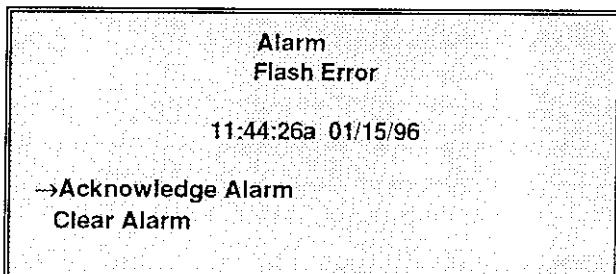
*NOTE: Clearing the alarm without correcting the problem that caused the alarm will cause the TCP to go into alarm condition displaying the pop up Alarm Screen.*
