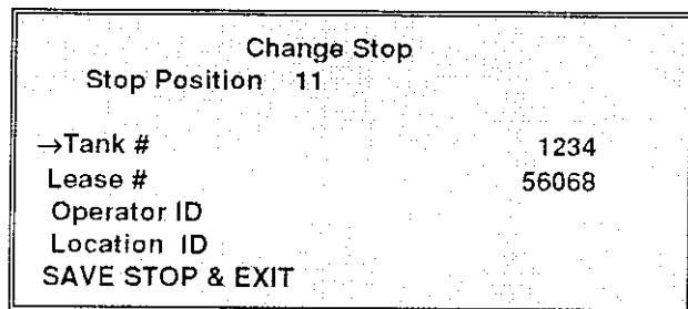
This screen shows the current stop information that is programmed. It indicates the stop position, the tank and lease number, and up to five additional items designated by the host. This information can be changed by going through the same steps that were described for adding a stop and when the information has been changed pressing "SAVE STOP & EXIT" and 'ENTER' to store the information in memory. If the information is not stored in memory the information will be lost.
