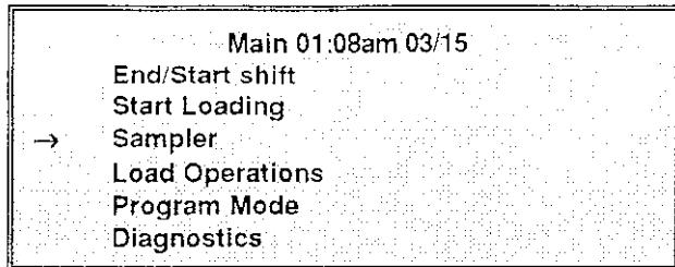
Pressing 'ENTER' with the cursor in front of "6 Sampler" displays the Sample Run Time Menu.
