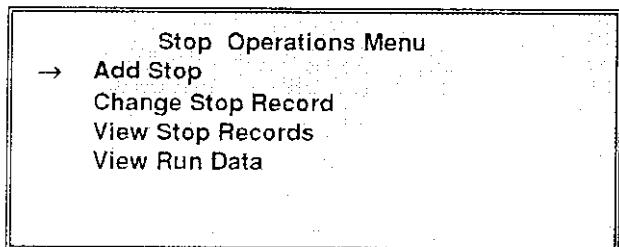
If there are no stop records set up for this truck, the only options that will be accessible on the menu will be "Add a Stop" or viewing of data.
