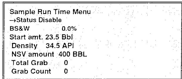
From the screen the sampler status and % BS&W can be changed. Information that is available for viewing only is the start amount, density, I/O point assigned to the sampler, the NSV product amount, total amount of product that has been taken (Total Grab) and the number of samples taken (Grab Count). The sampler start amount can be changed in the program mode.
