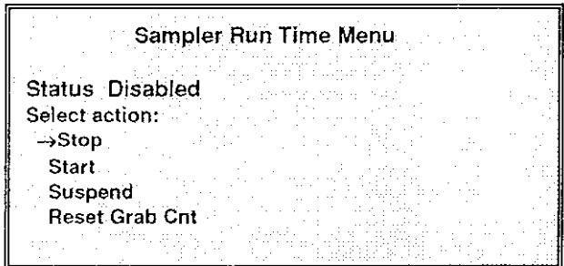
From the screen the operator can start, stop or suspend or reset the grab count of the sampler.
