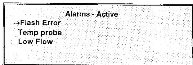
Up to six active alarms will be displayed on the Active Alarm screen. With the cursor in front of the alarm that is to be cleared pressing 'ENTER' will bring up a pop up screen.
