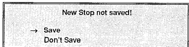
When either is selected and the 'ENTER' key is pressed the TCP will revert back to the "Stop Operations Menu". If 'CLEAR' is pressed the unit will revert back to the stop definition screen.
