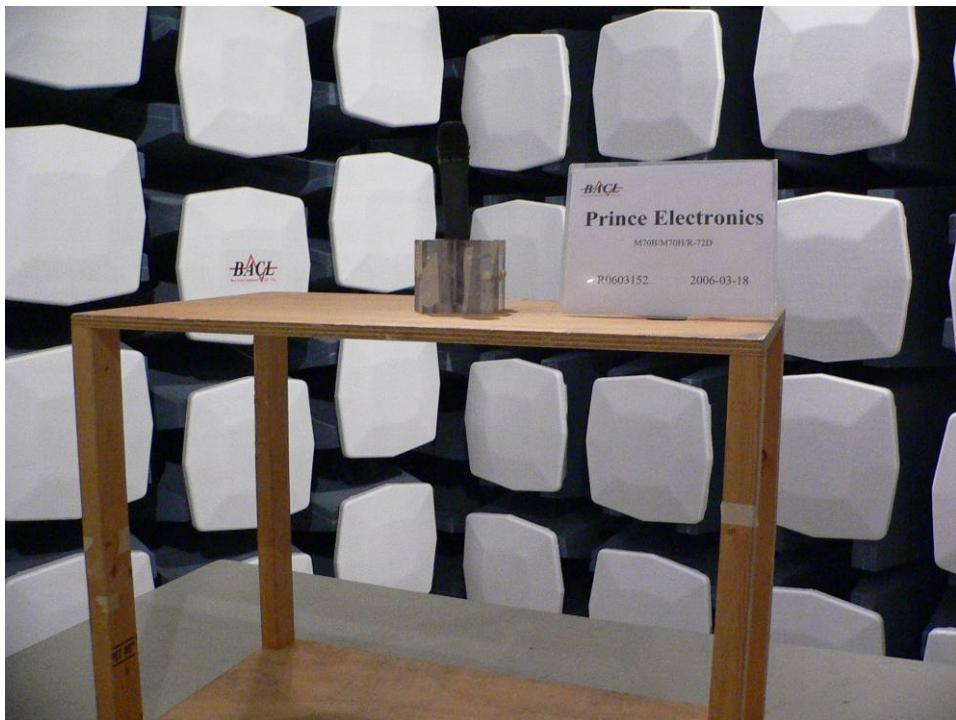
**Radiated Emission - Rear View (M-70H)**
