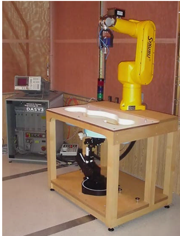
DASY3 SAR Measurement System
