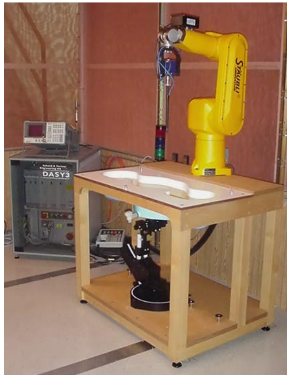
DASY3 SAR Measurement System
