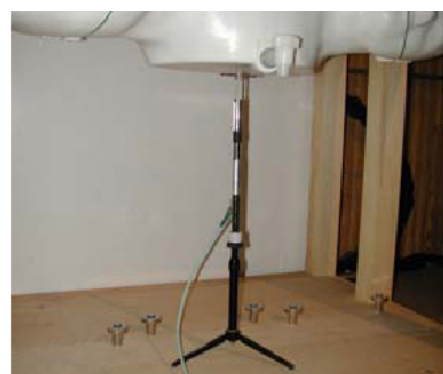
Figure 12.1 Dipole Validation Test Setup
