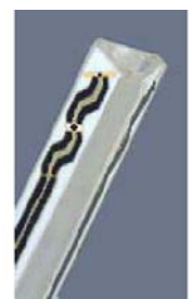
Figure 3.2 Probe Thick-Film Technique
