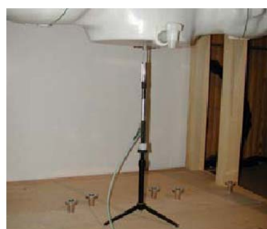
Figure 12.1 Dipole Validation Test Setup
