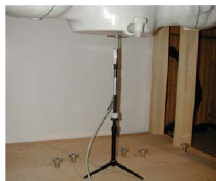
Figure 12.1 Dipole Validation Test Setup
