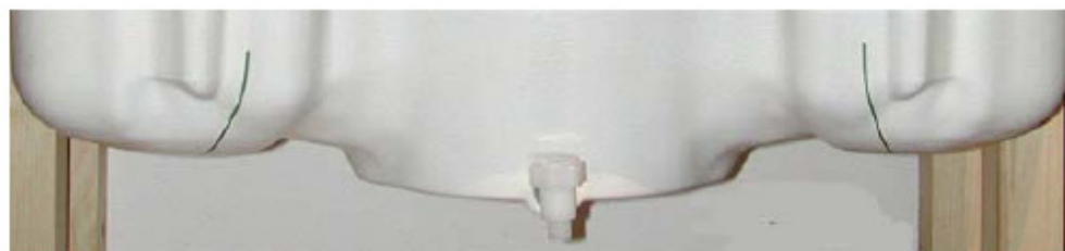
Figure 7.2 SAM Twin Phantom shell
