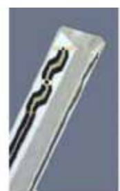
Figure 3.2 Probe Thick-Film Technique
