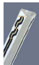
Figure 3.2 Probe Thick-Film Technique
