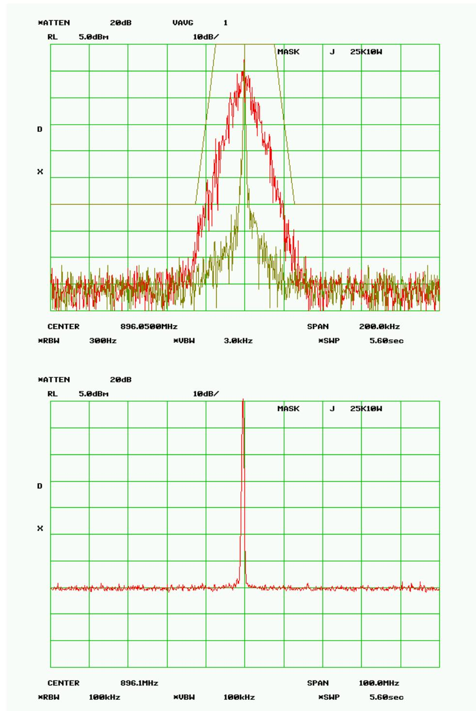
**MASK J - 25 kHz - 1.0 Watts****RF Frequency 896.050 MHz****SPECTRUM FOR EMISSION - 17K8F1D**
