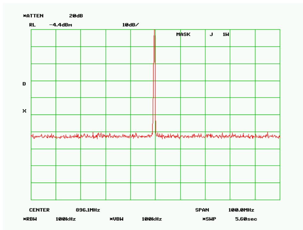
**MASK J - 10 Watts****RF Frequency 896.050 MHz****SPECTRUM FOR EMISSION - 8K08F1D**
