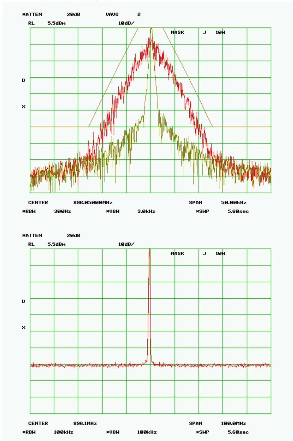
**MASK J - 1.0 Watt****RF Frequency 896.050 MHz****SPECTRUM FOR EMISSION - 8K50F1D**
