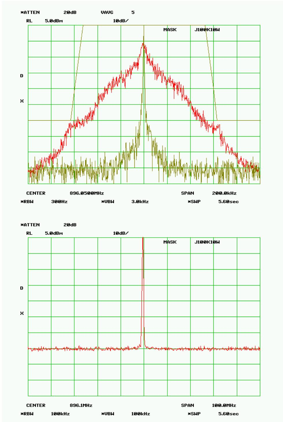
**MASK J - 100 kHz - 1.0 Watts****RF Frequency 896.050 MHz****SPECTRUM FOR EMISSION - 49K7F1D**
