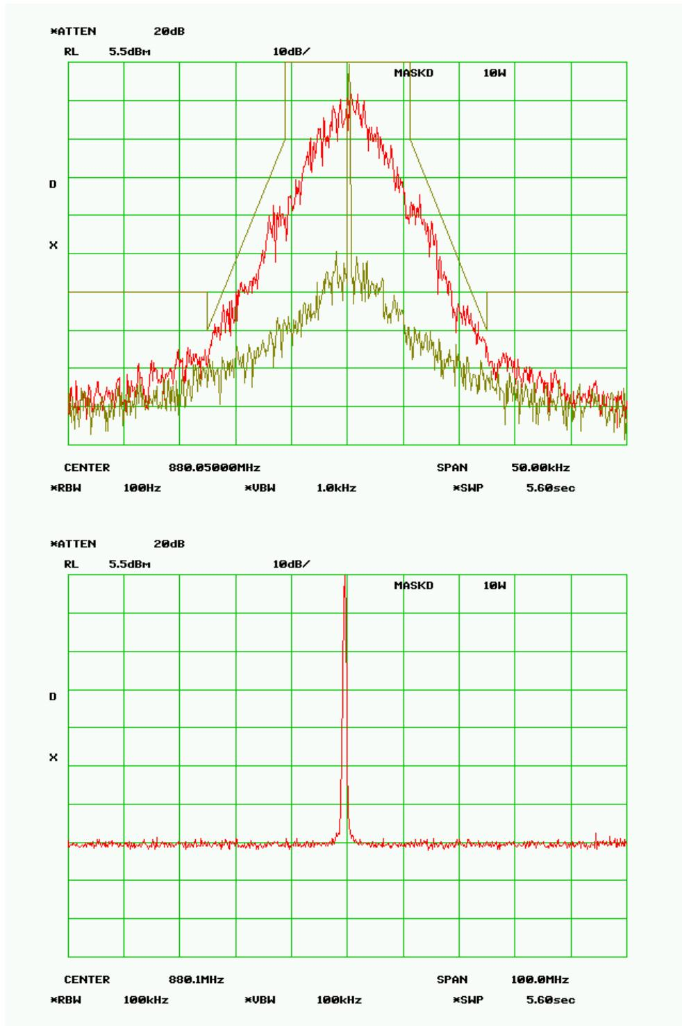
**MASK D - 1.0 Watt****RF Frequency 880.050 MHz****SPECTRUM FOR EMISSION - 8K30F1D**
