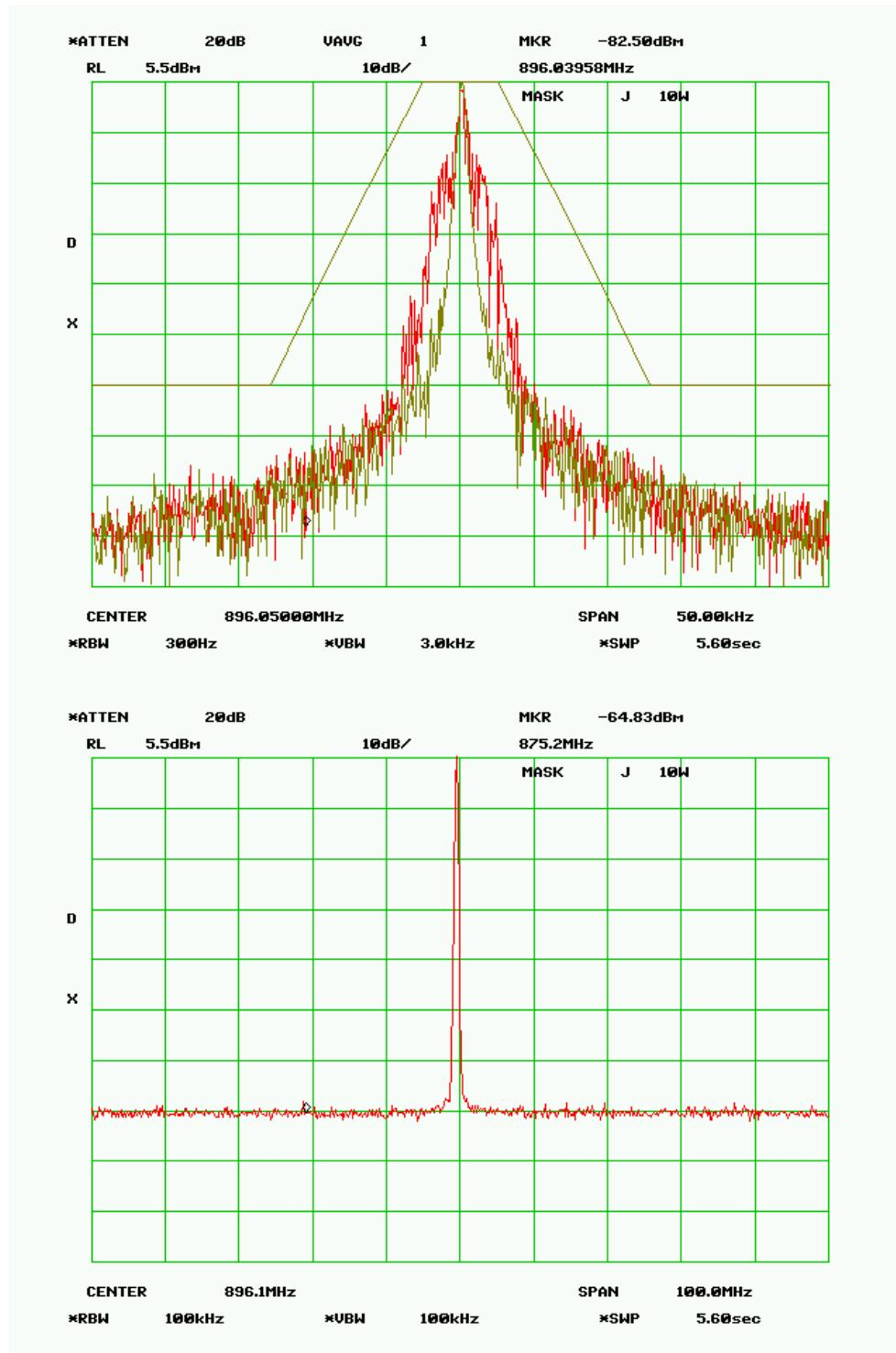
**MASK J – 1.0 Watts****RF Frequency 896.050 MHz****SPECTRUM FOR EMISSION - 3K20F1D**
