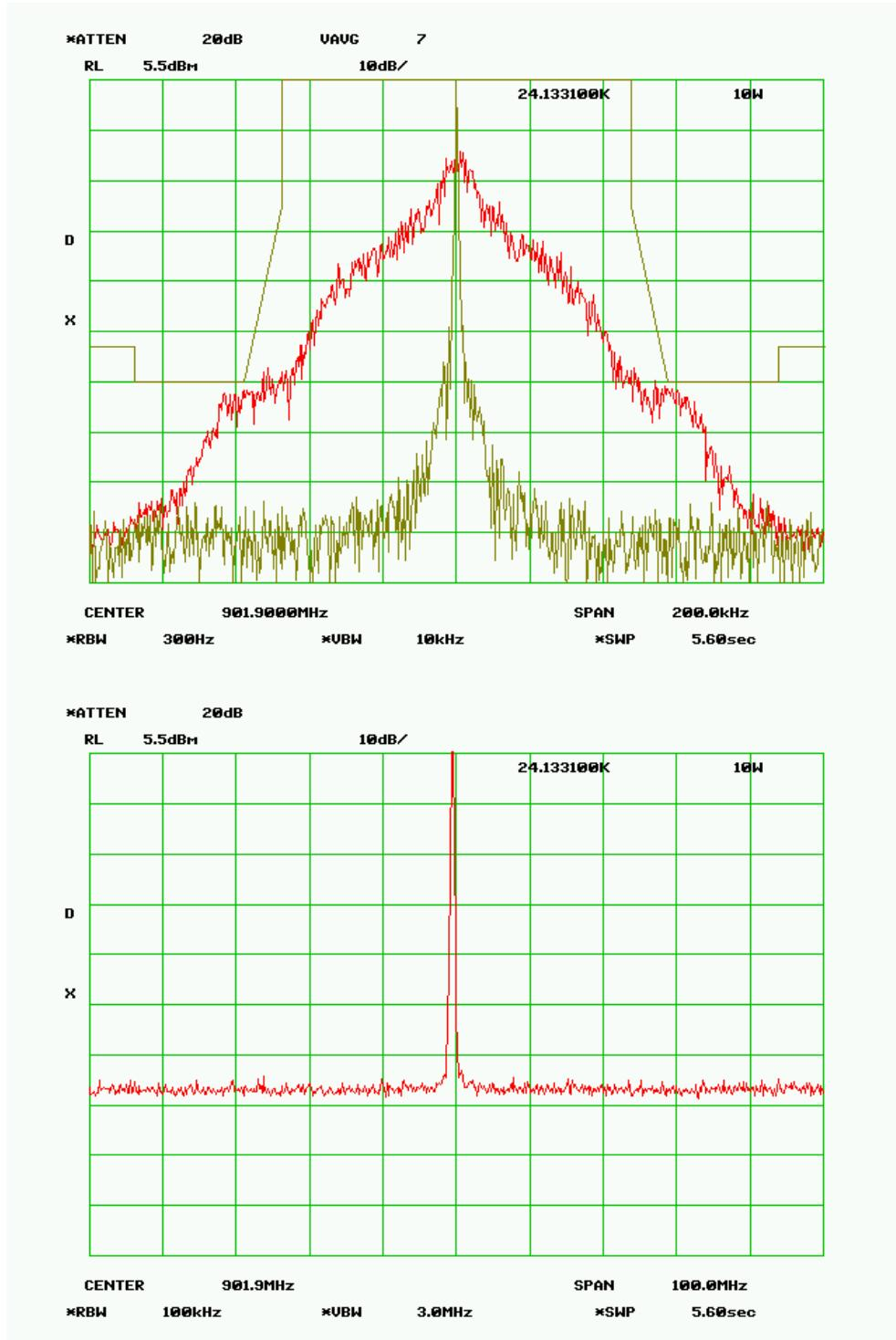
**MASK 24.133a1 - 100 kHz - 1.0 Watts****RF Frequency 901.900****SPECTRUM FOR EMISSION - 52K7F1D**
