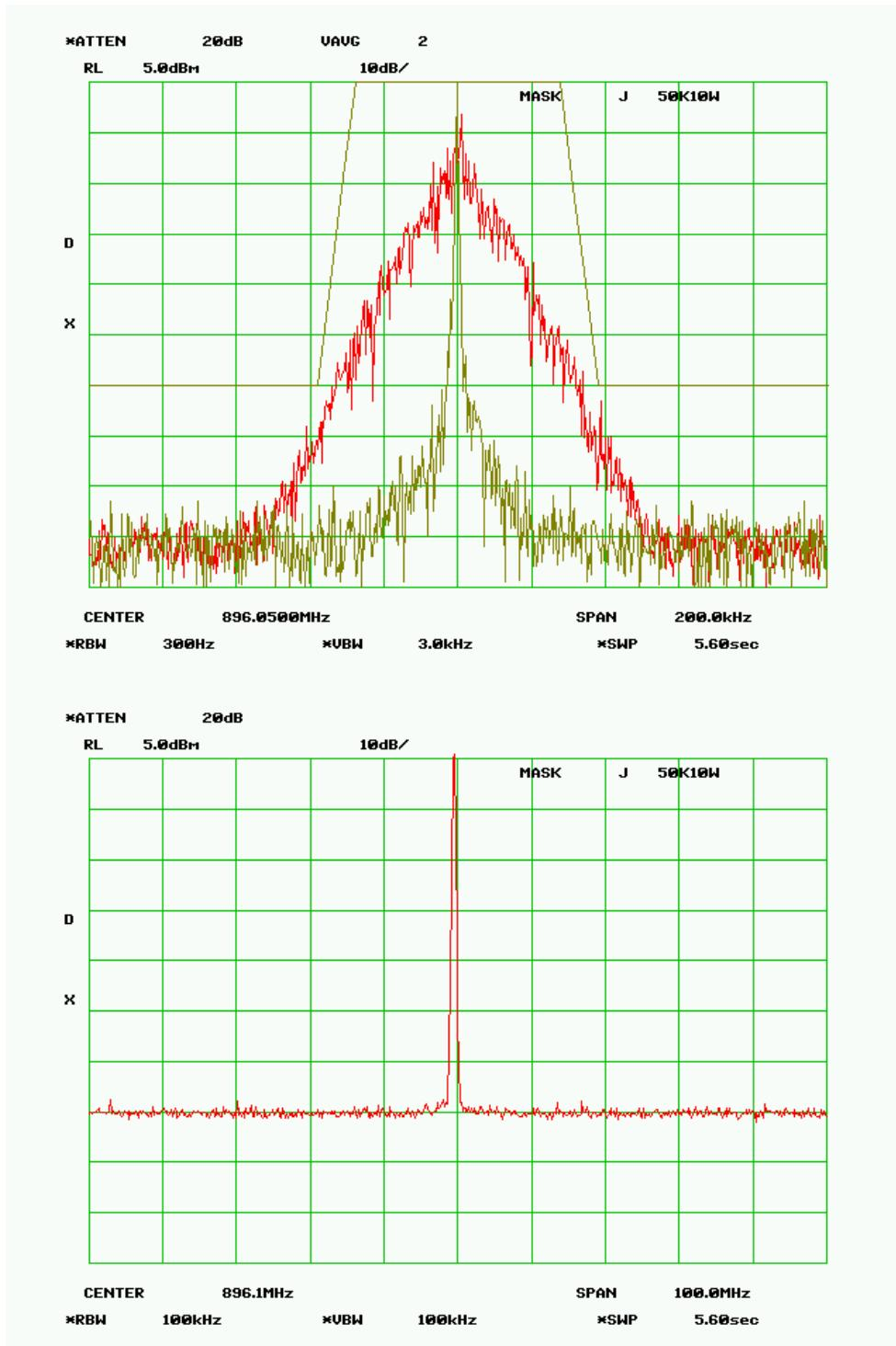
**MASK J - 50 kHz - 1.0 Watts****RF Frequency 896.050 MHz****SPECTRUM FOR EMISSION - 29K5F1D**
