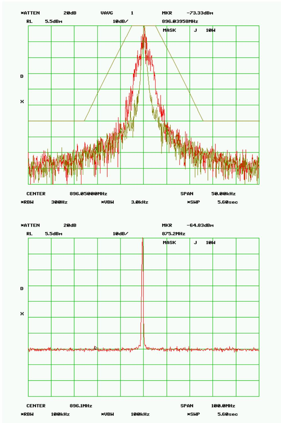
**MASK J - 1.0 Watt****RF Frequency 896.050 MHz****SPECTRUM FOR EMISSION - 8K20F1D**
