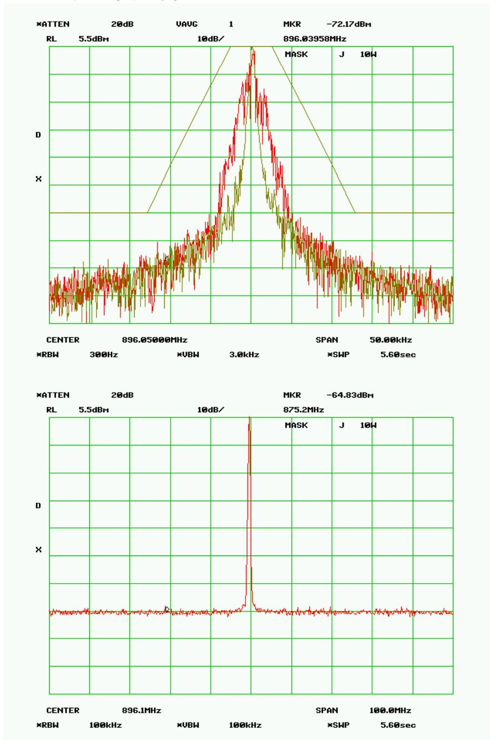
**MASK J – 1.0 Watts****RF Frequency 896.050 MHz****SPECTRUM FOR EMISSION - 3K55F1D**
