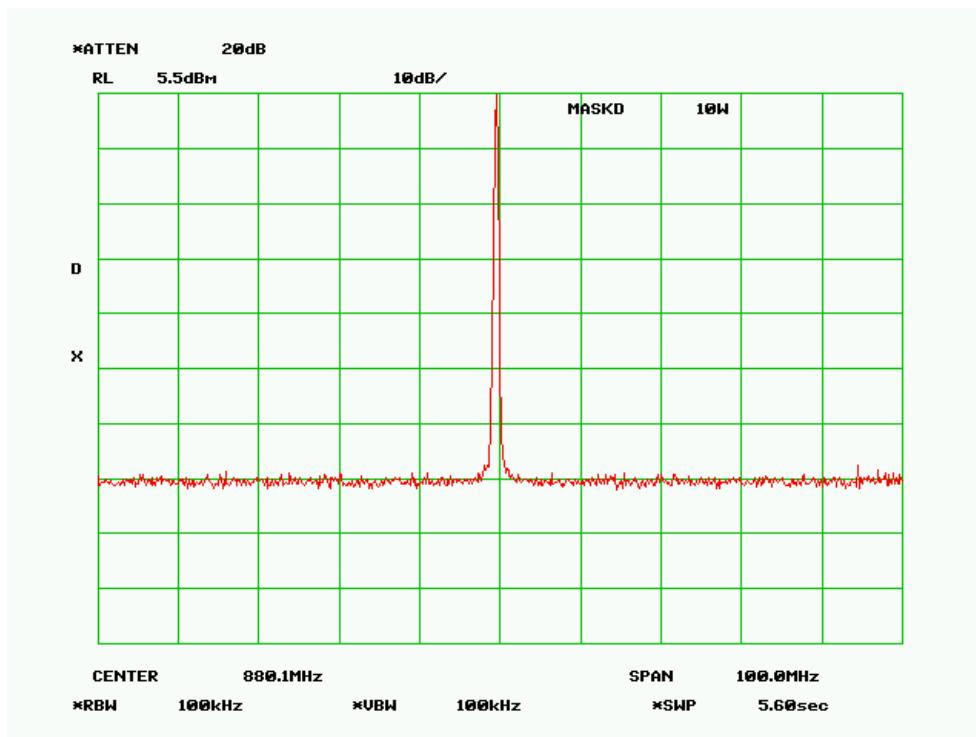
**MASK D - 1.0 Watt****RF Frequency 880.050 MHz****SPECTRUM FOR EMISSION - 8K50F1D**
