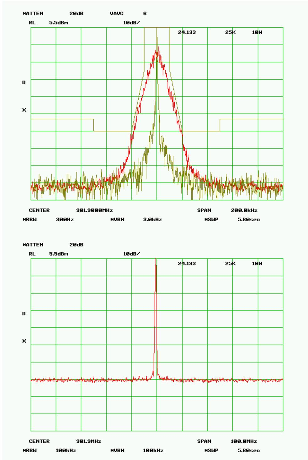
**MASK 24.133a1 - 25 kHz - 1.0 Watts****RF Frequency 901.900****SPECTRUM FOR EMISSION - 17K8F1D**
