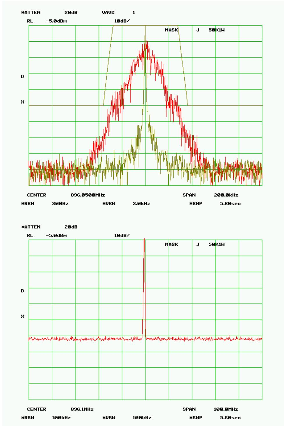
**MASK J - 50 kHz - 10.0 Watts****RF Frequency 896.050 MHz****SPECTRUM FOR EMISSION - 29K8F1D**
