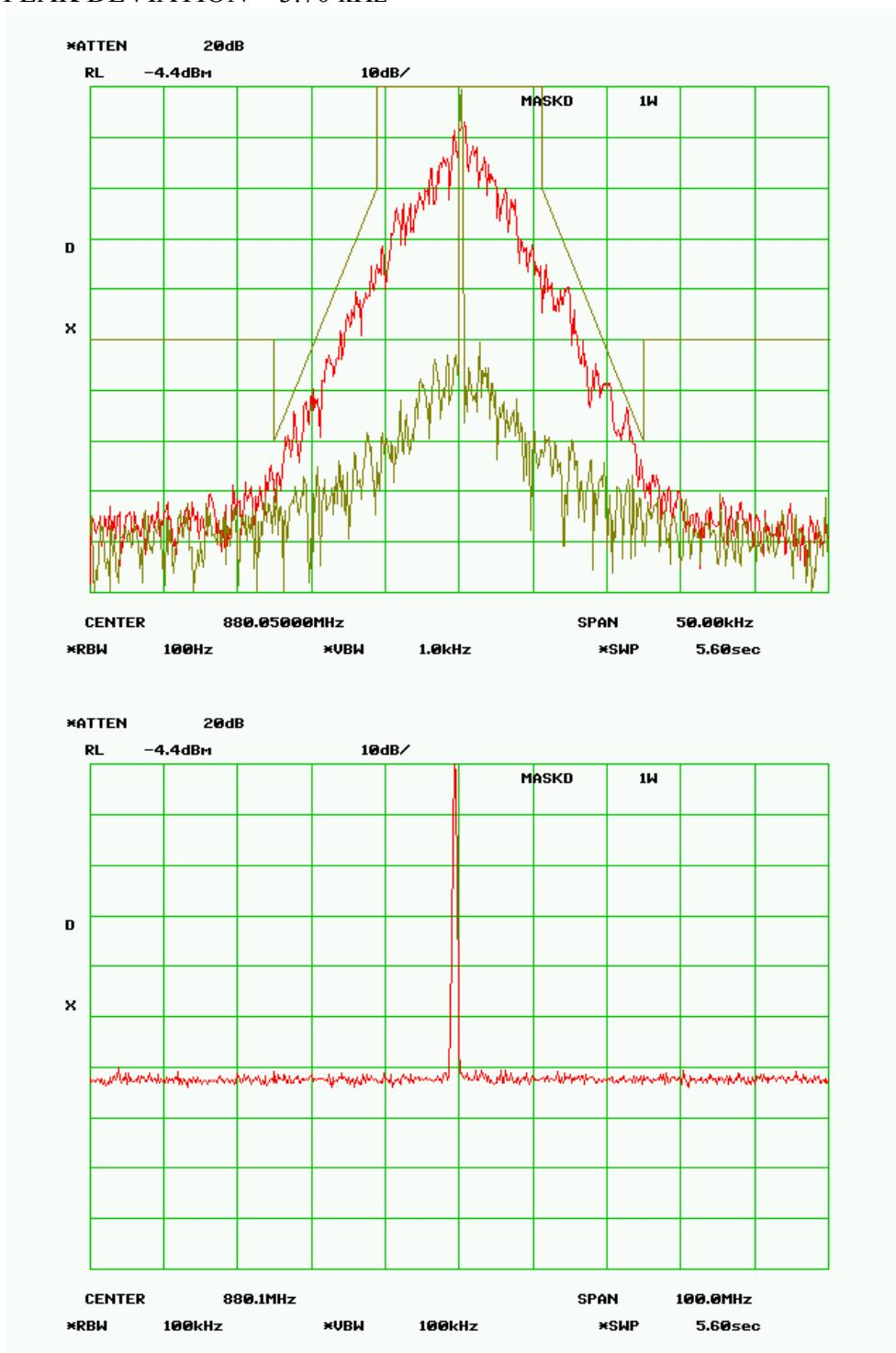
**MASK D - 10 Watts****RF Frequency 880.050 MHz****SPECTRUM FOR EMISSION - 8K30F1D**
