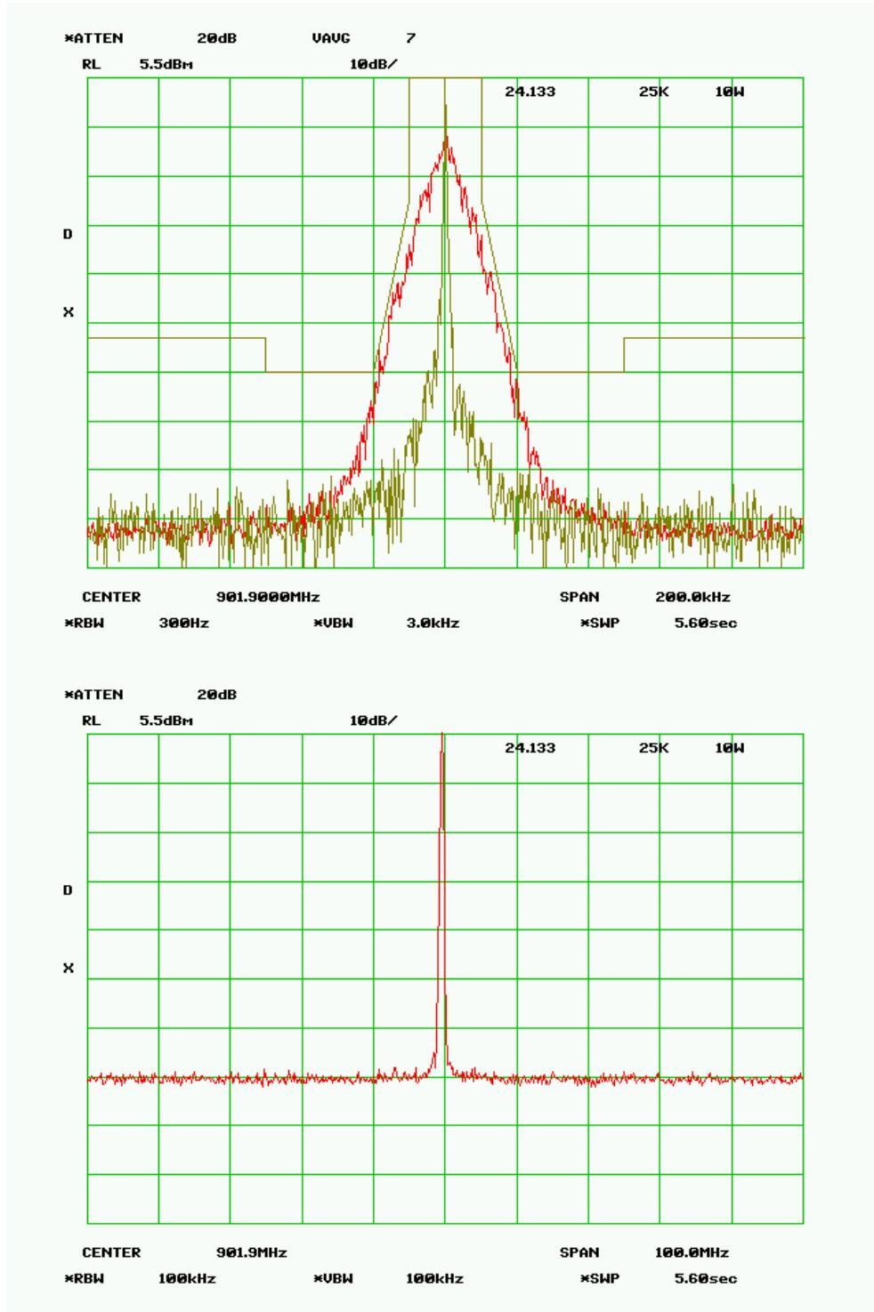
**MASK 24.133a1 - 25 kHz - 1.0 Watts**
