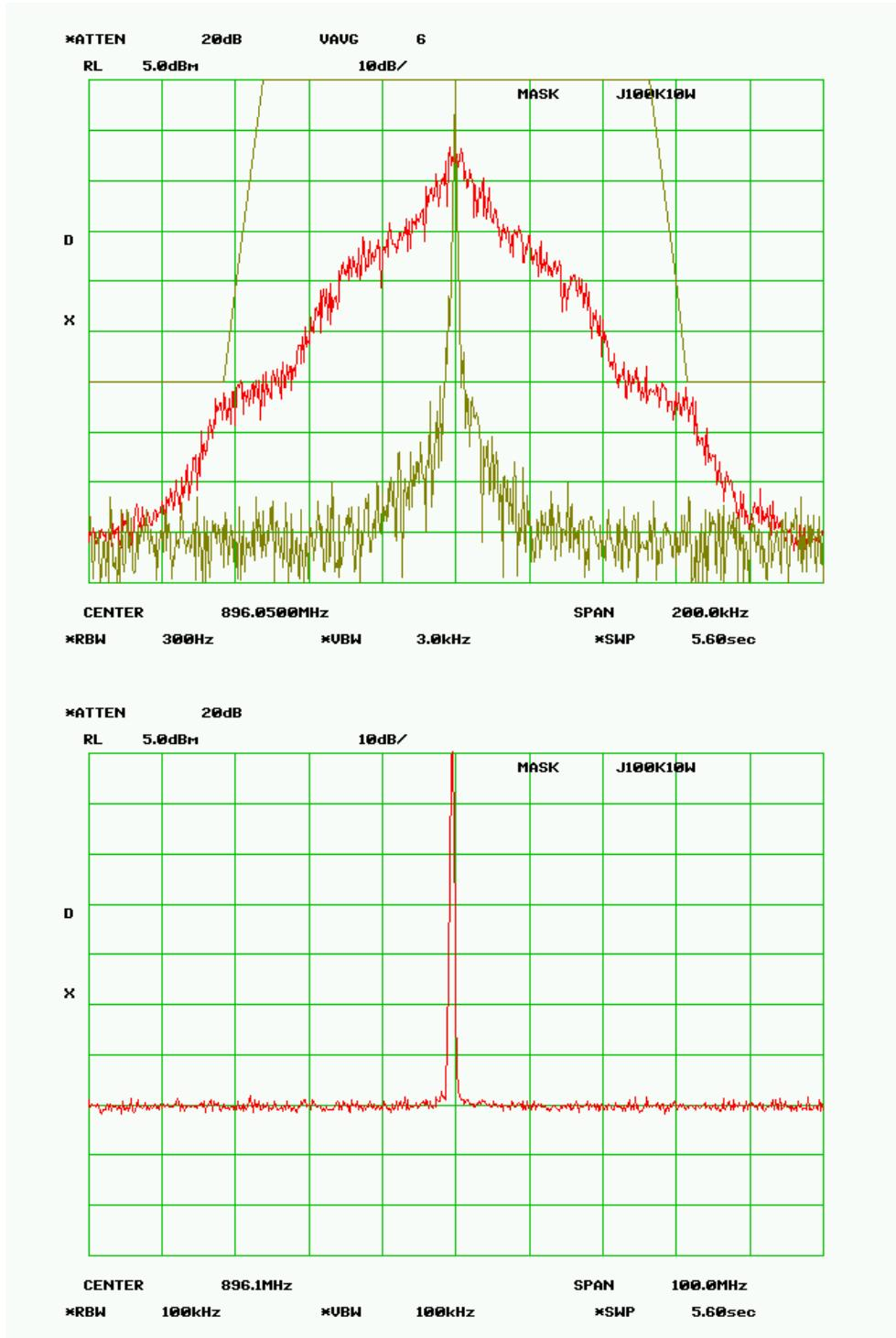
**MASK J - 100 kHz - 1.0 Watts****RF Frequency 896.050 MHz****SPECTRUM FOR EMISSION - 52K7F1D**
