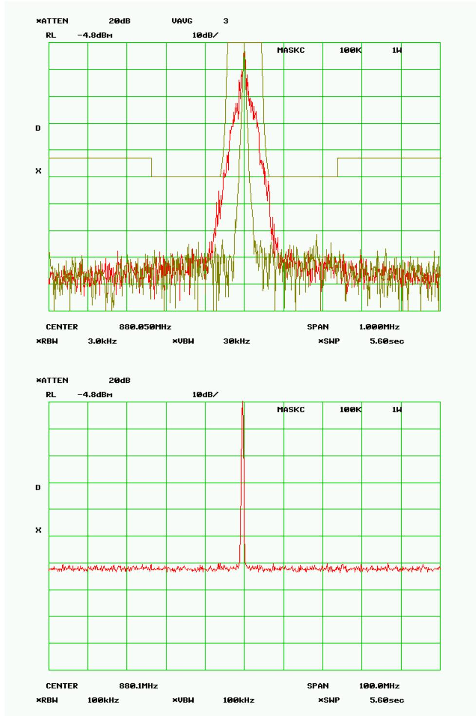
**MASK C - 10 Watts****RF Frequency 880.050 MHz****SPECTRUM FOR EMISSION - 51K3F1D**
