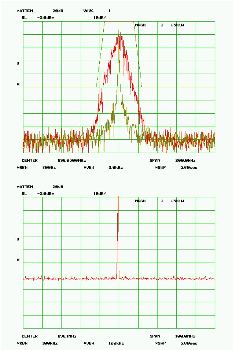
**MASK J - 25 kHz - 10.0 Watts****RF Frequency 896.050 MHz****SPECTRUM FOR EMISSION - 17K8F1D**
