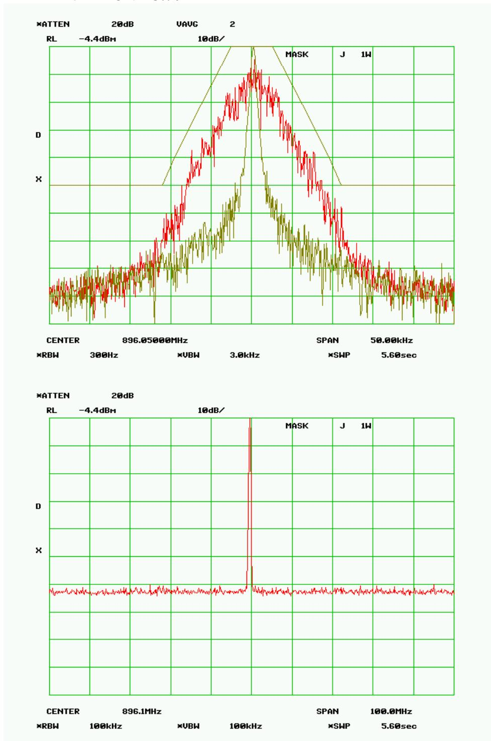
**MASK J - 10 Watts****RF Frequency 896.050 MHz****SPECTRUM FOR EMISSION - 8K30F1D**
