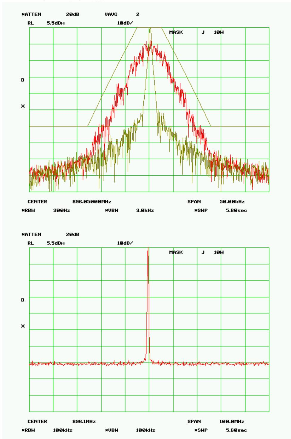
**MASK J - 1.0 Watt****RF Frequency 896.050 MHz****SPECTRUM FOR EMISSION - 8K30F1D**
