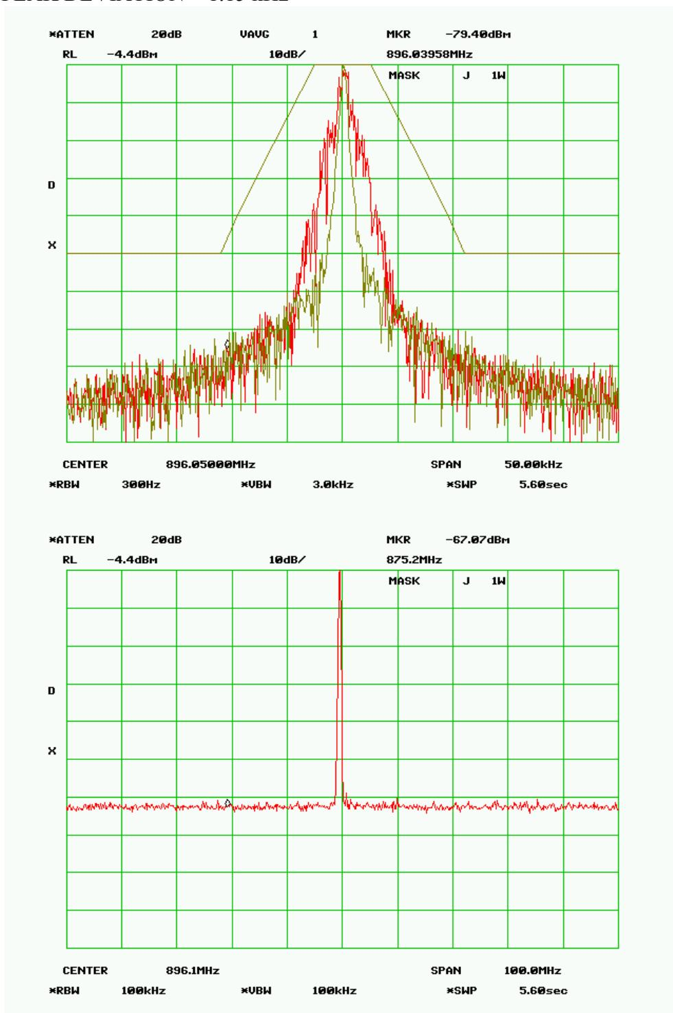
**MASK J – 10.0 Watts****RF Frequency 896.050 MHz****SPECTRUM FOR EMISSION - 3K30F1D**
