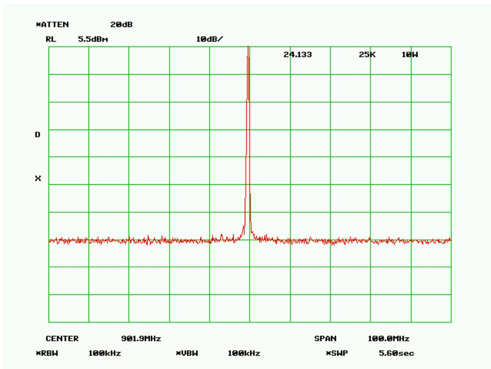
**MASK 24.133a1 - 25 kHz - 1.0 Watts****RF Frequency 901.900****SPECTRUM FOR EMISSION - 16K8F1D**
