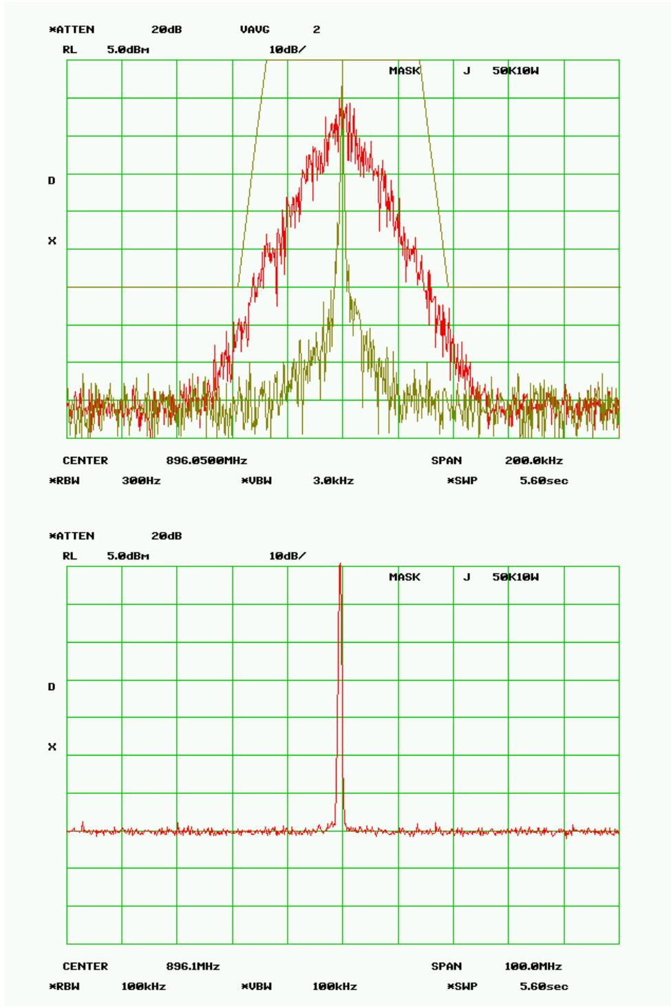
**MASK J - 50 kHz - 1.0 Watts****RF Frequency 896.050 MHz****SPECTRUM FOR EMISSION - 30K5F1D**
