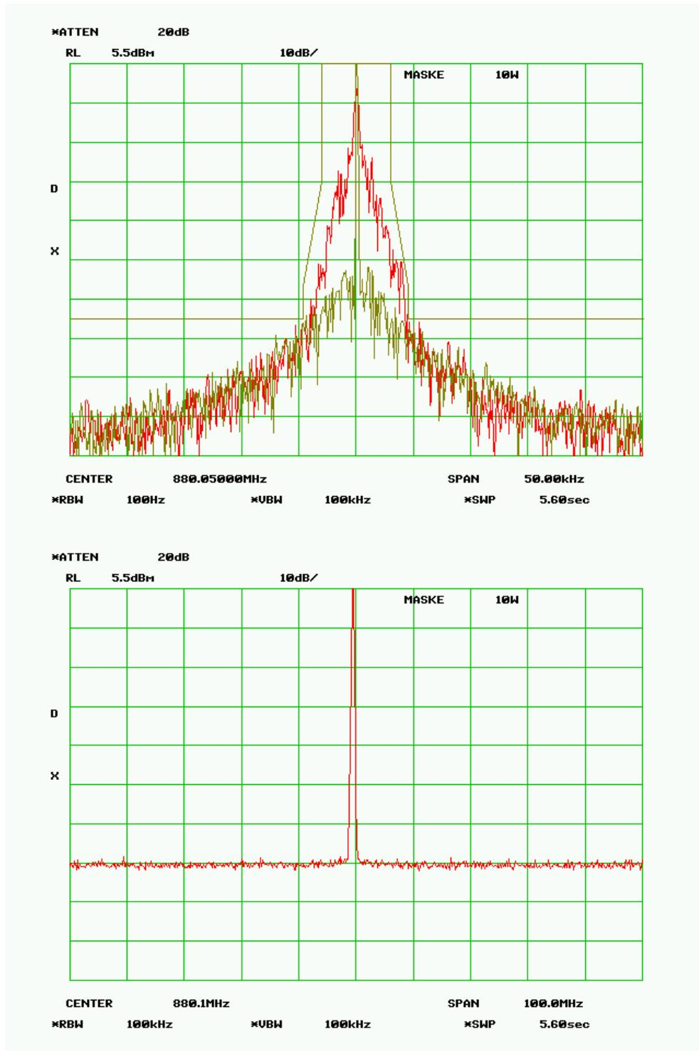
**MASK E – 1.0 Watts****RF Frequency 880.050 MHz****SPECTRUM FOR EMISSION - 3K20F1D**
