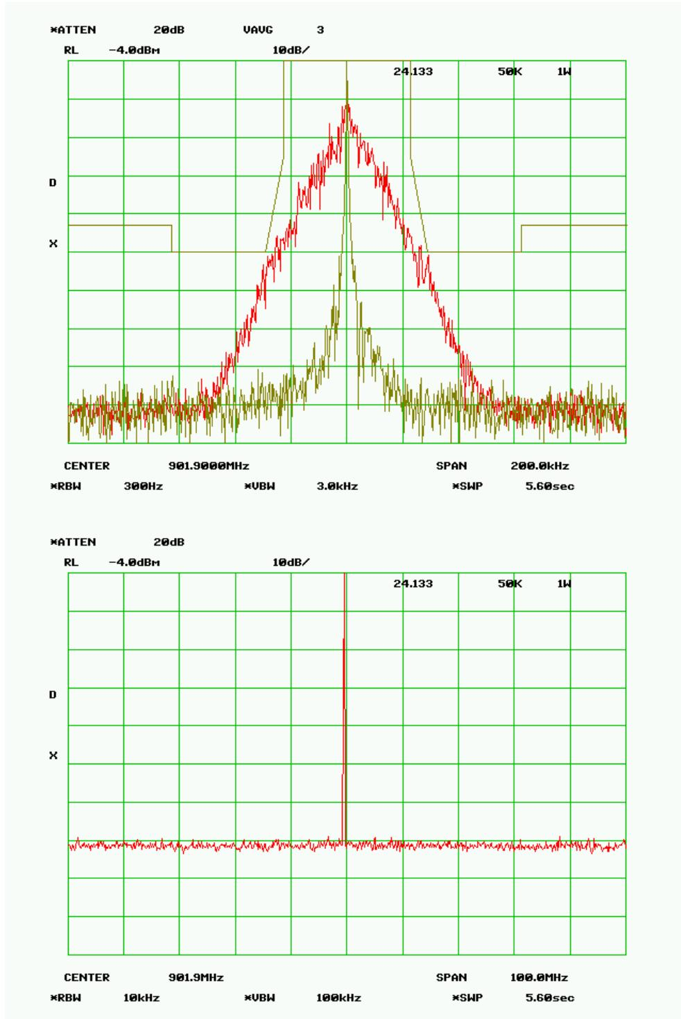
**MASK 24.133a1 - 50 kHz - 10.0 Watts**
