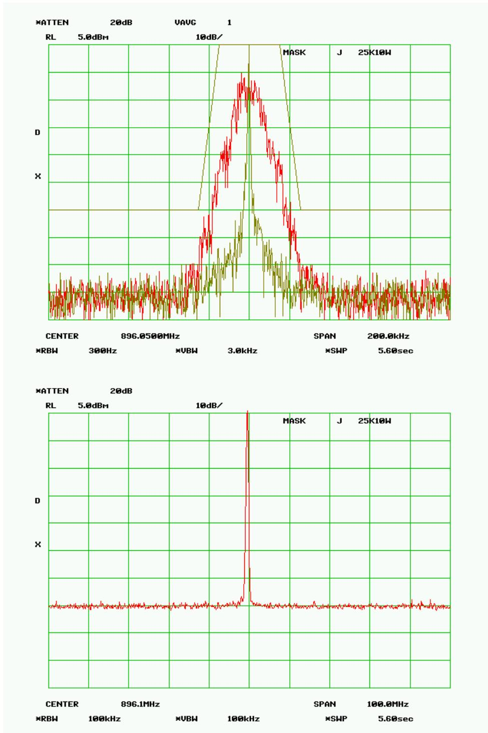
**MASK J - 25 kHz - 1.0 Watts****RF Frequency 896.050 MHz****SPECTRUM FOR EMISSION - 16K8F1D**
