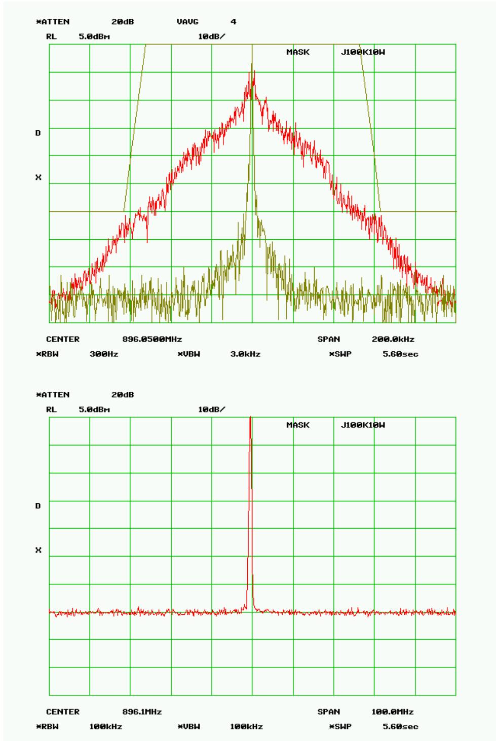
**MASK J - 100 kHz - 1.0 Watts****RF Frequency 896.050 MHz****SPECTRUM FOR EMISSION - 51K3F1D**
