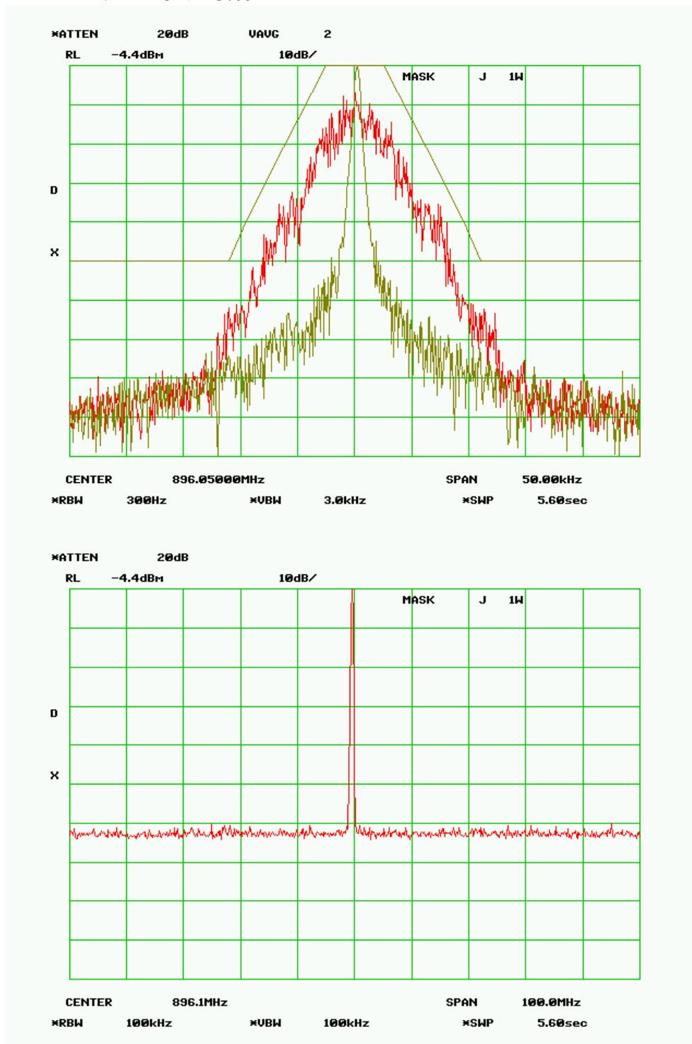
**MASK J - 10 Watts****RF Frequency 896.050 MHz****SPECTRUM FOR EMISSION - 8K20F1D**
