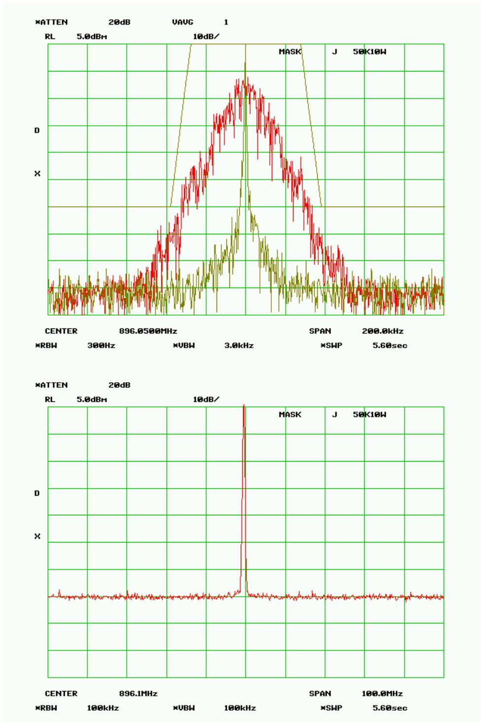
**MASK J - 50 kHz - 1.0 Watts****RF Frequency 896.050 MHz****SPECTRUM FOR EMISSION - 30K0F1D**
