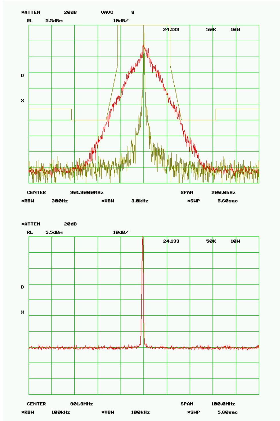
**MASK 24.133a1 - 50 kHz - 1.0 Watts**
