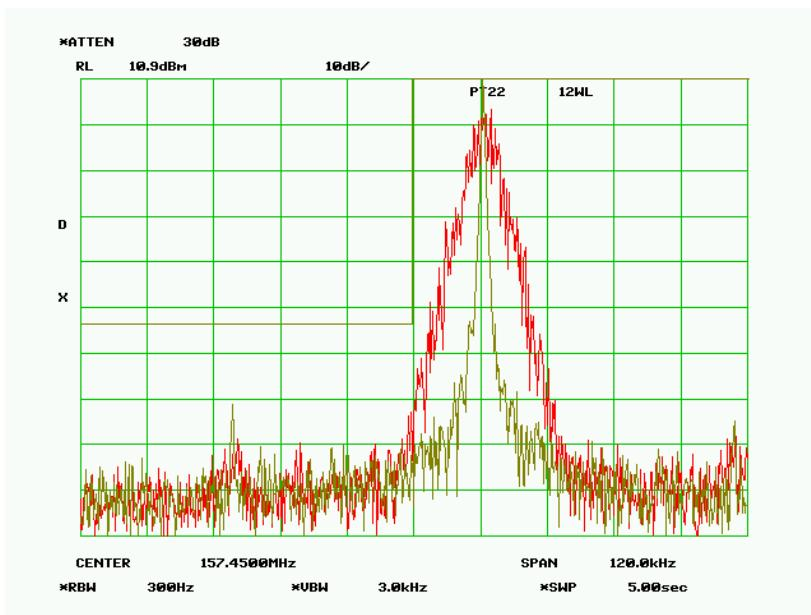
**Band Edge – 157.450000, Test Frequency - 157.462500 MHz**
