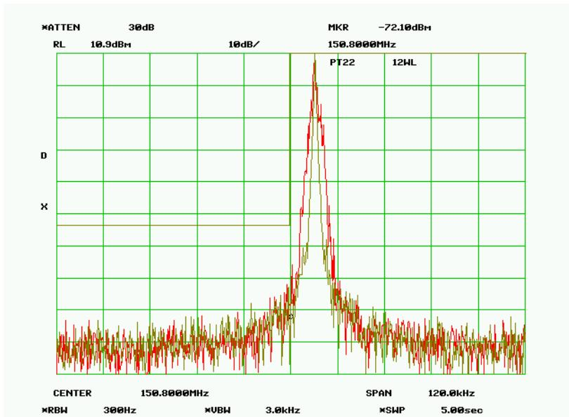
**Band Edge – 150.800000 Test Frequency - 150.806250 MHz**
