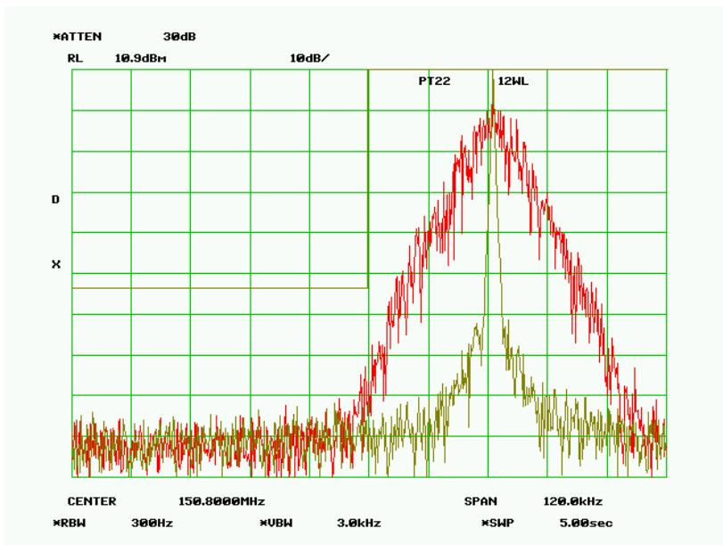
**Band Edge – 157.450000, Test Frequency - 157.456250 MHz**
