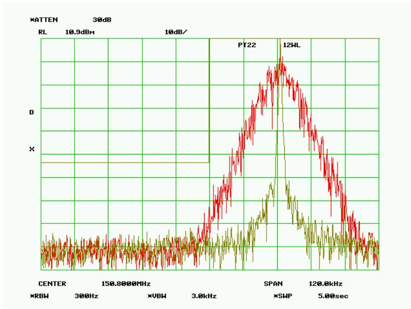
**Band Edge – 150.800000, Test Frequency - 150.825000 MHz**
