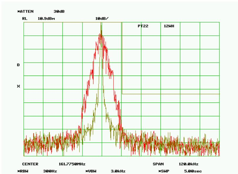
**Band Edge – 161.775000, Test Frequency – 161.762500 MHz**
