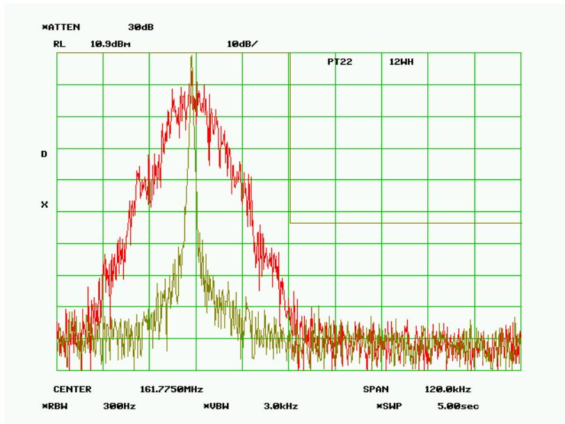
**Band Edge – 161.775000, Test Frequency – 161.750000 MHz**
