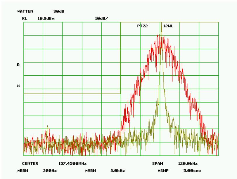
**Band Edge – 157.450000, Test Frequency - 157.475000 MHz**
