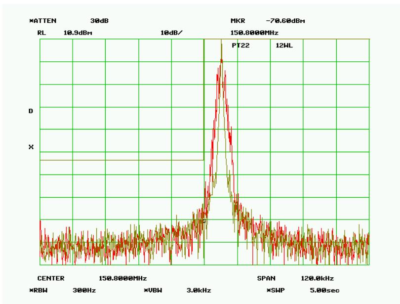
**Band Edge – 150.800000, Test Frequency - 150.812500 MHz**
