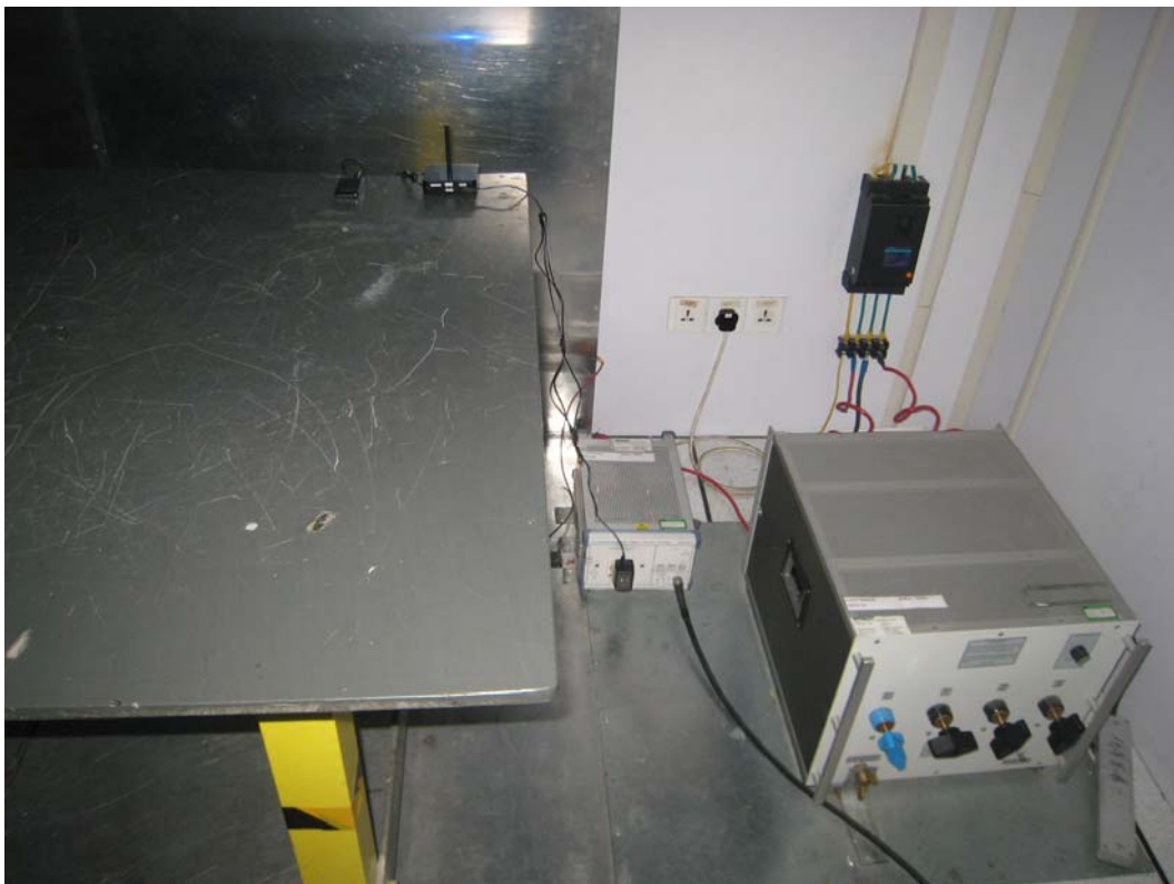
Conducted Emission Test Setup
