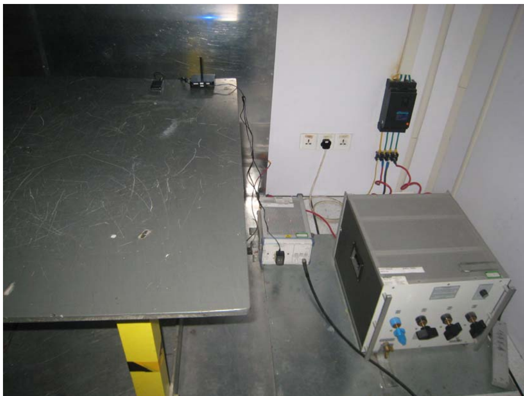
Conducted Emission Test Setup
