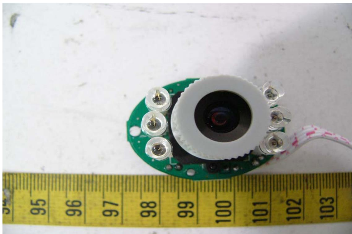
10. Solder View of CCD's PCB
