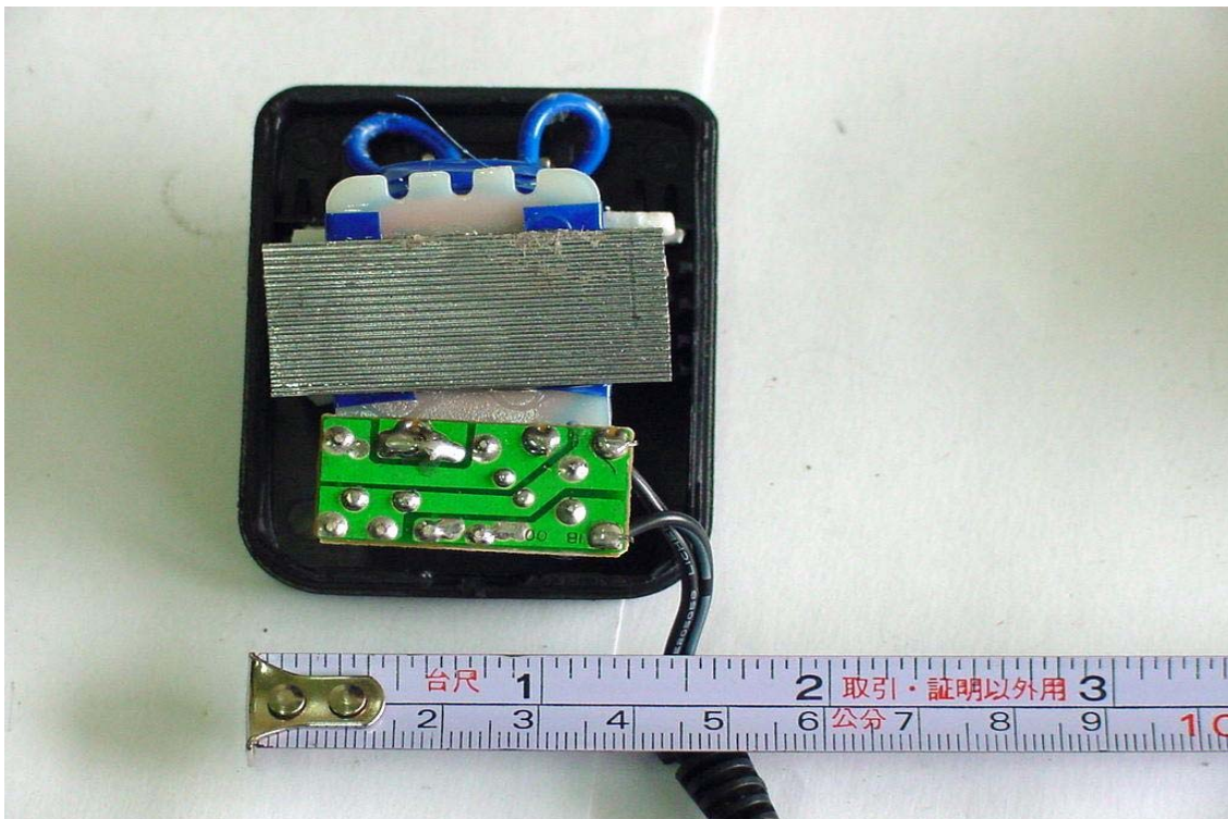
Solder View of Adaptor's PCB
