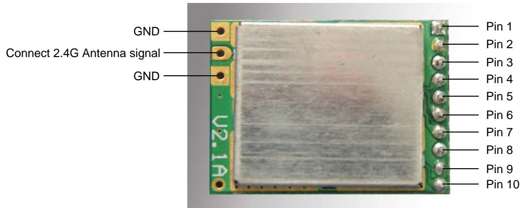
Pin 1: Power supply voltage +5V.
