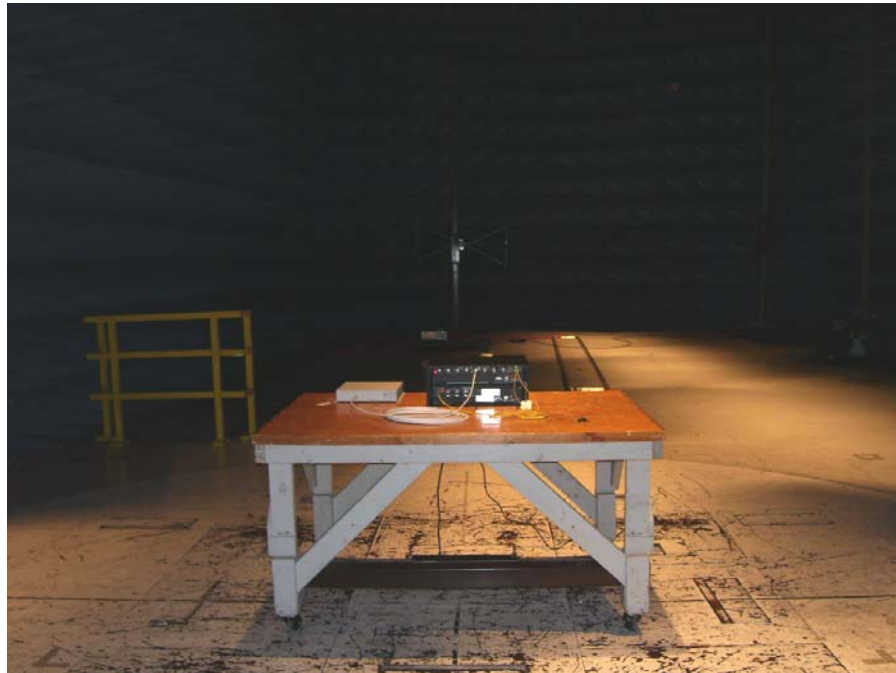
Photograph 5. Radiated Emission Limits Test Setup, 30 MHz to 1 GHz, Front View
