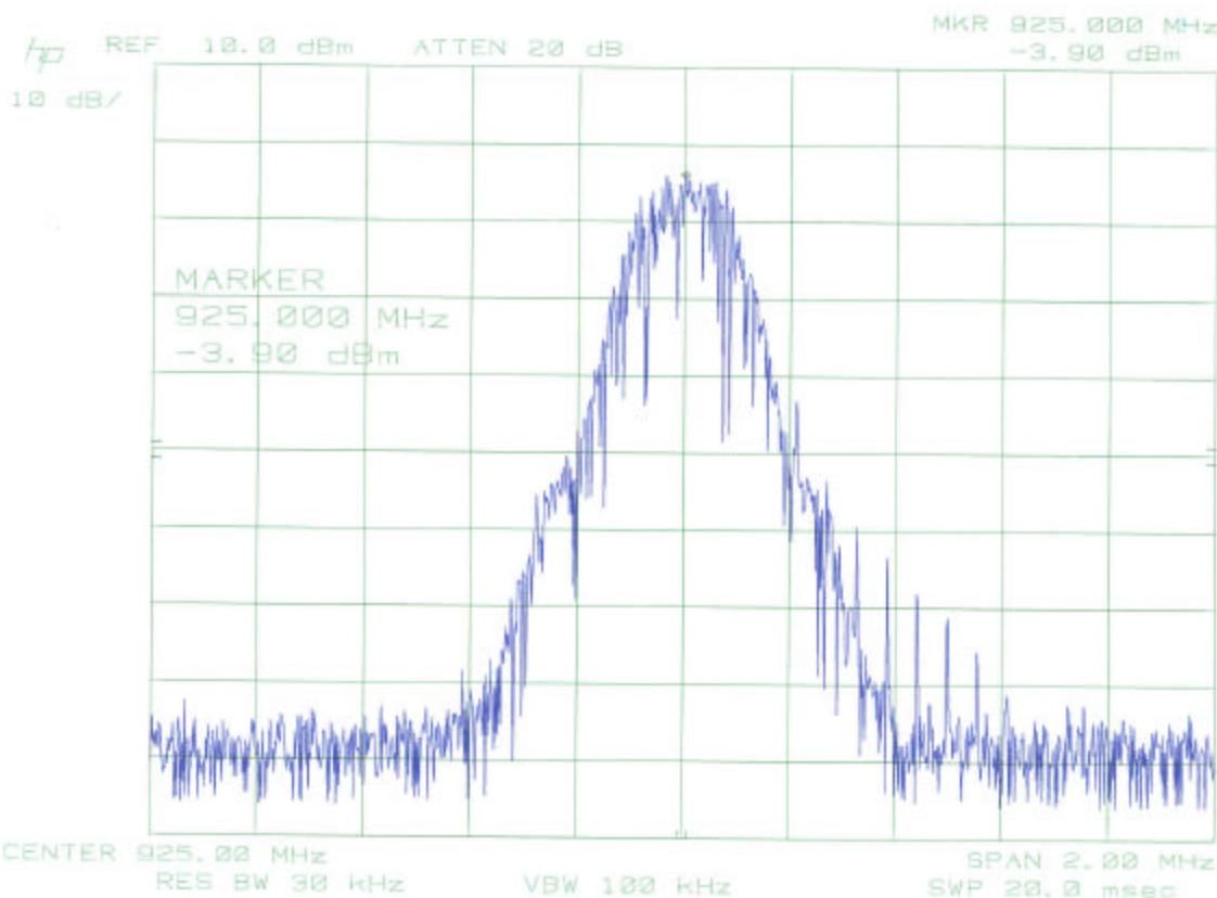
**Occupied Bandwidth – Downlink****925.000 MHz- Signal Generator**
