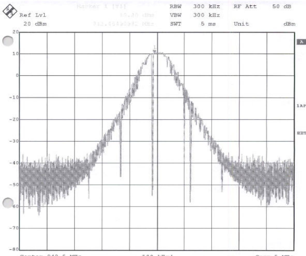
**Occupied Bandwidth – Downlink****942.500 MHz- Signal Generator**
