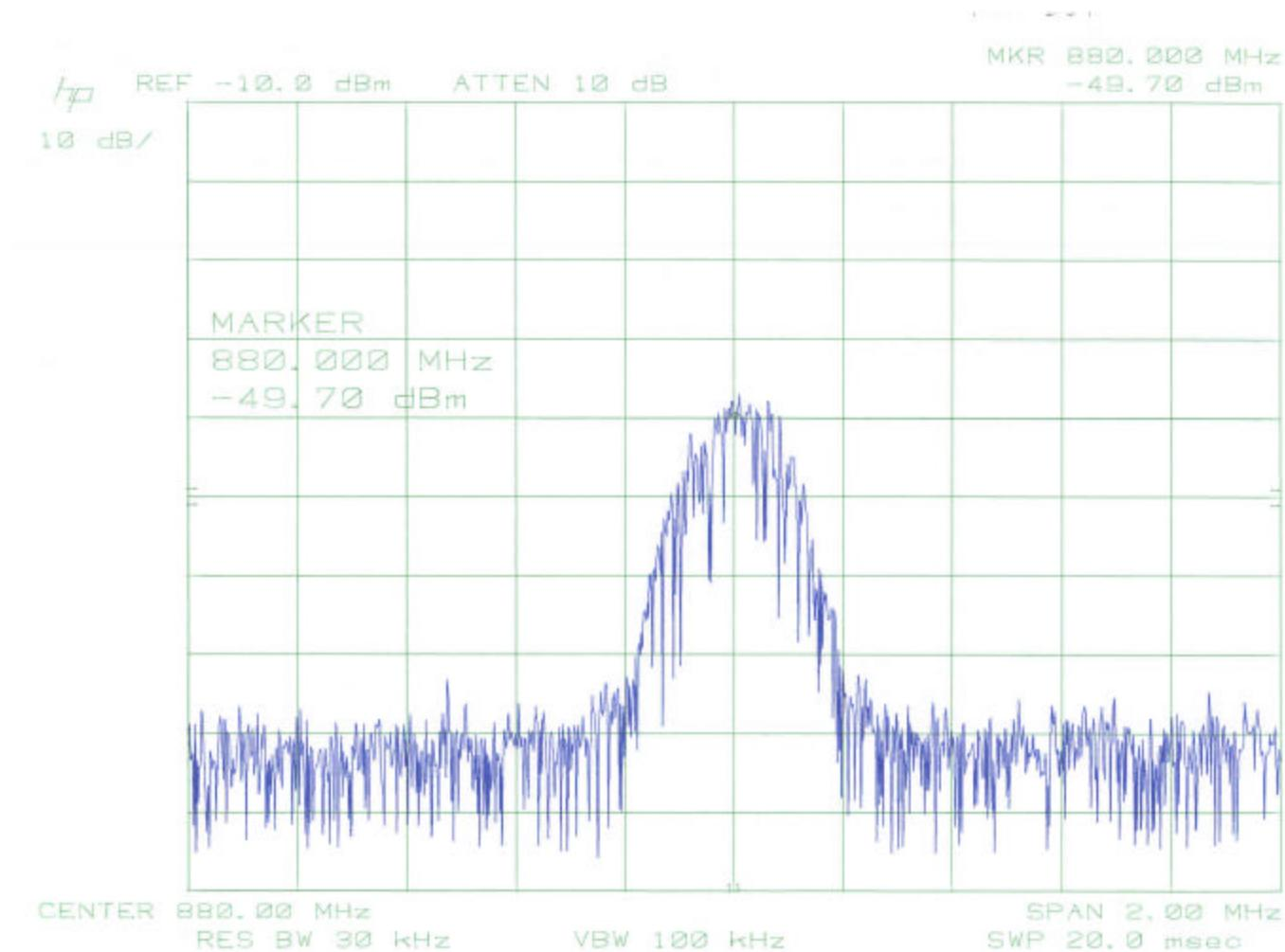
**Occupied Bandwidth – Uplink****880.000 MHz – Signal Generator**
