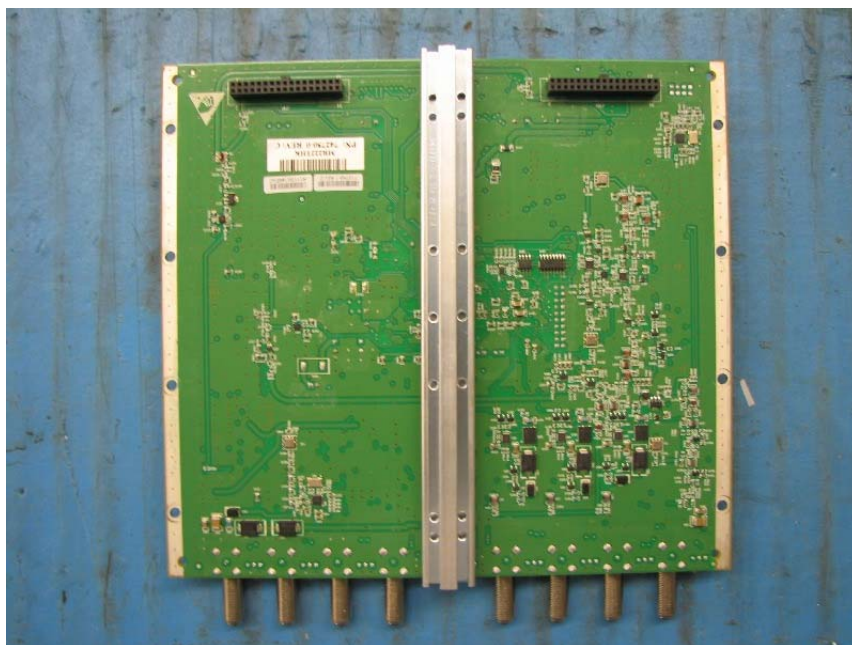
PCB IF Assembly Top View - MRAU
