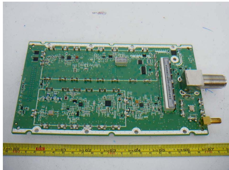
**13.22 EUT 1900 MHz PCS Band Module – Main PCB Board Solder View**
