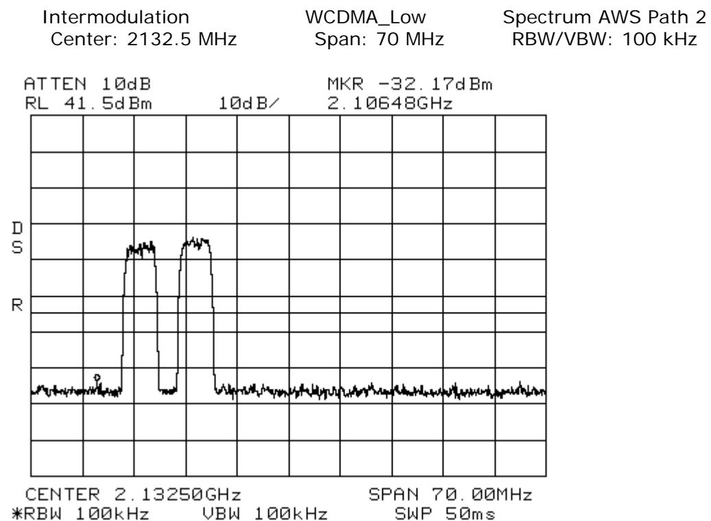
Intermodulation WCDMA\_Low Spectrum AWS Path 2
