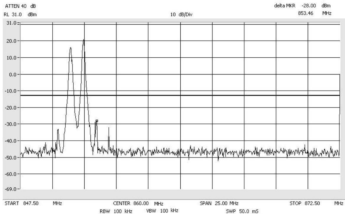
Intermodulation      iDEN\_Low      SMR\_800\_MHz
