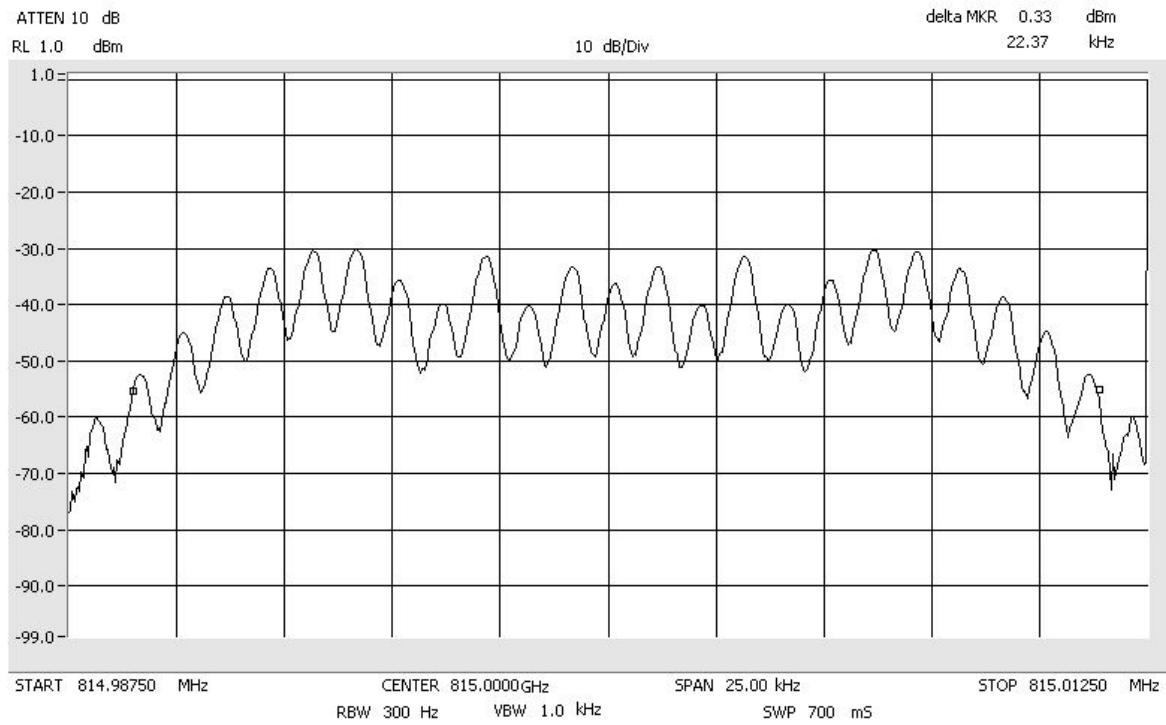
Occupied Bandwidth iDEN\_Signal\_In
