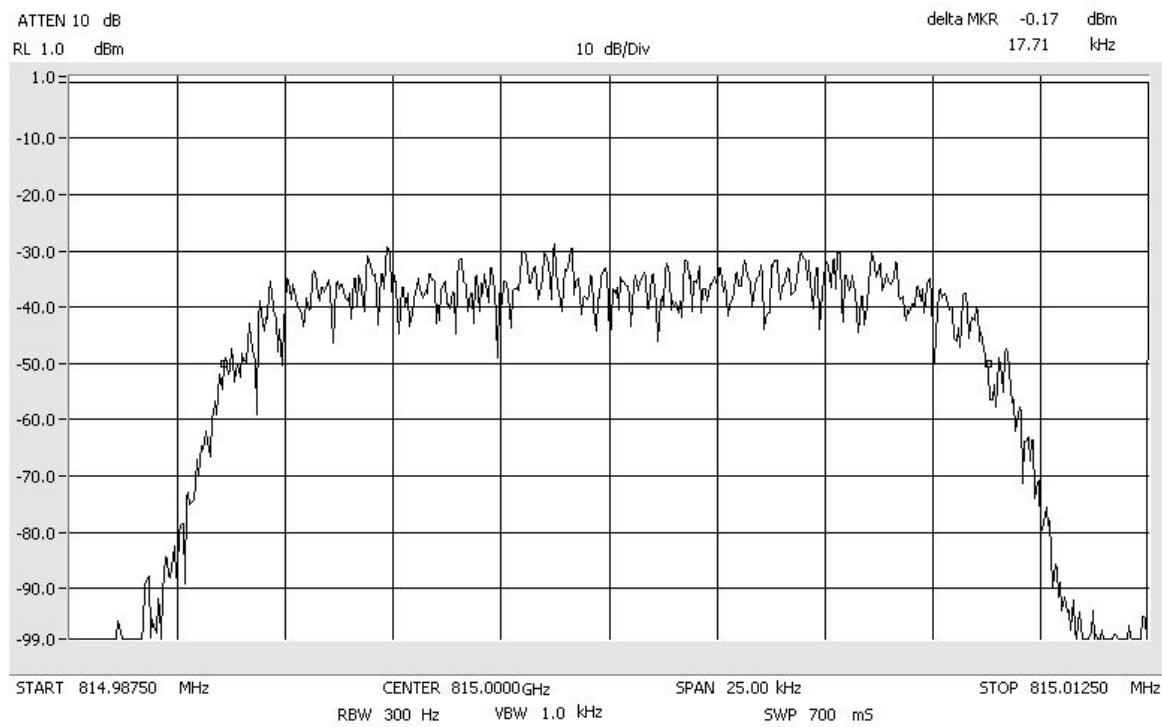
Occupied Bandwidth iDEN\_Signal\_Out
