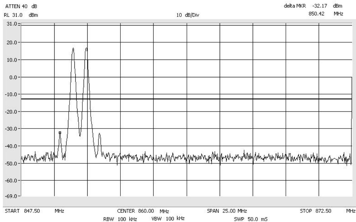
Intermodulation      FM\_Low      SMR\_800\_MHz
