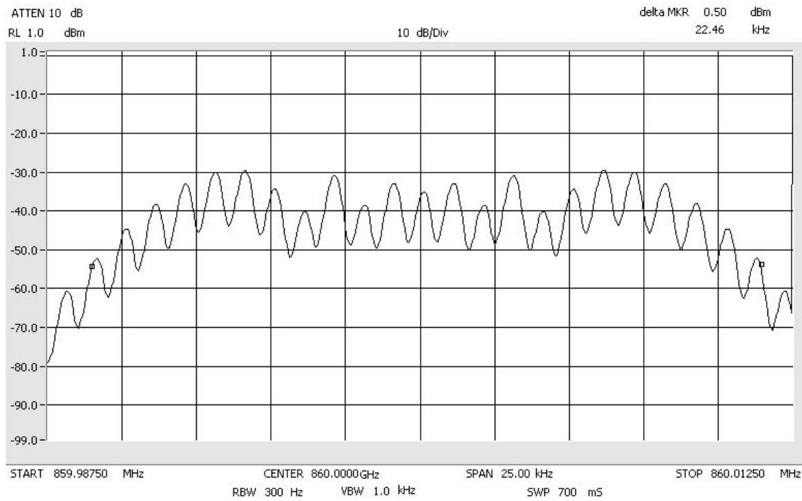
Occupied Bandwidth FM\_Signal\_Out
