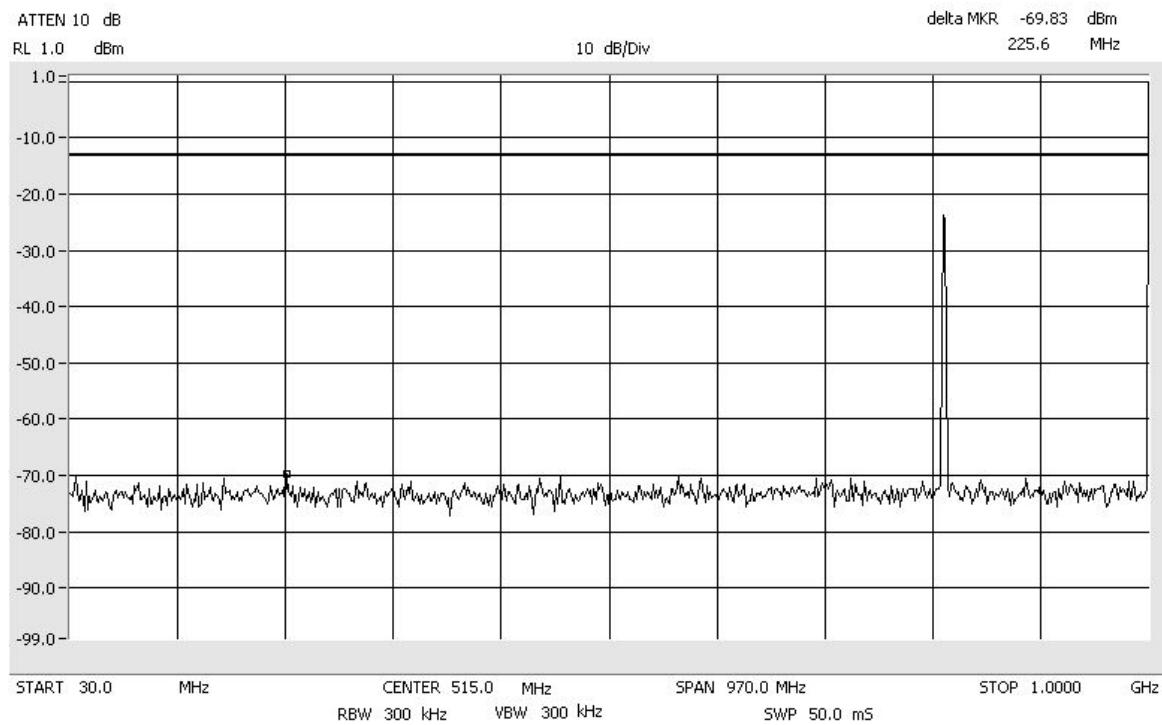
Intermodulation iDEN\_High SMR\_800\_MHz
