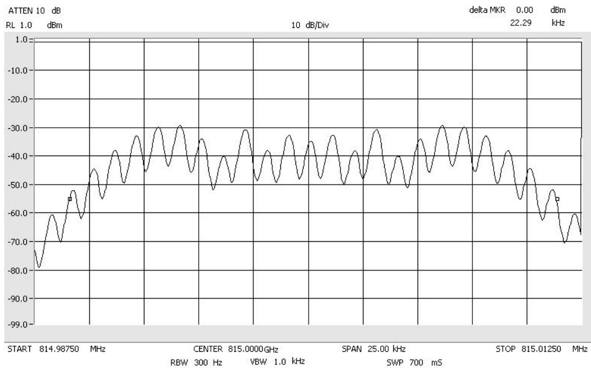
Occupied Bandwidth FM\_Signal\_Out
