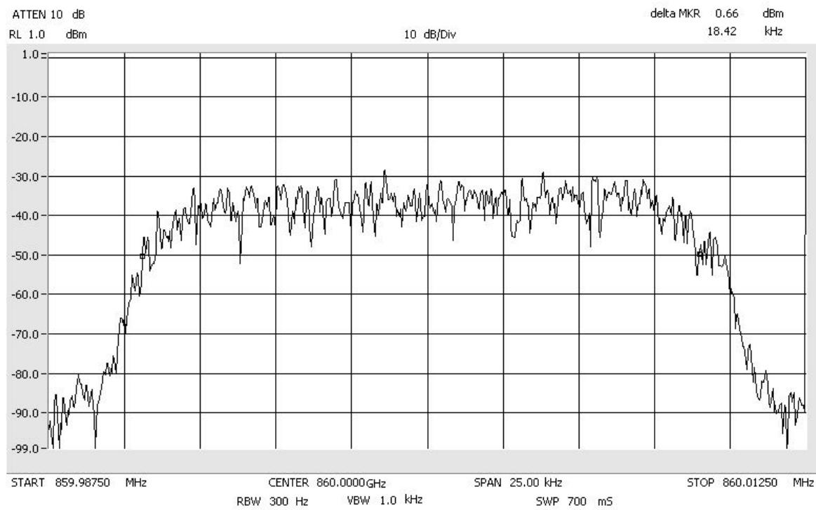
Occupied Bandwidth iDEN\_Signal\_Out
