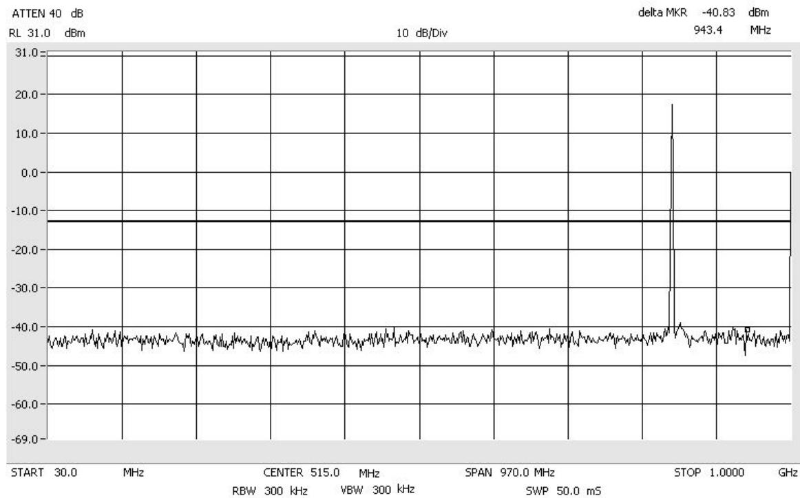
Intermodulation APCO25\_C4FM\_Low SMR\_800\_MHz
