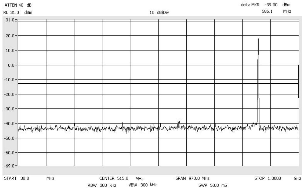
Intermodulation APCO25\_CQPSK\_High SMR\_800\_MHz
