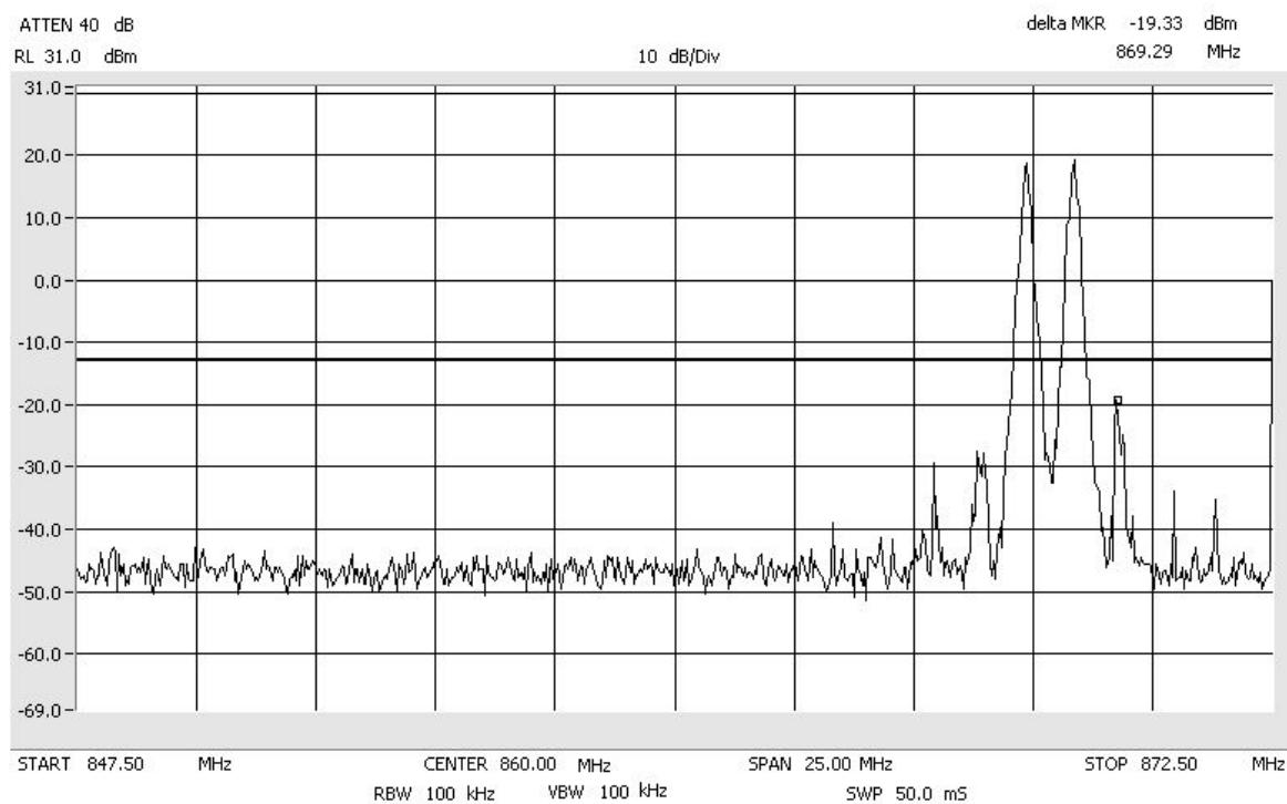
Intermodulation      iDEN\_High      SMR\_800\_MHz
