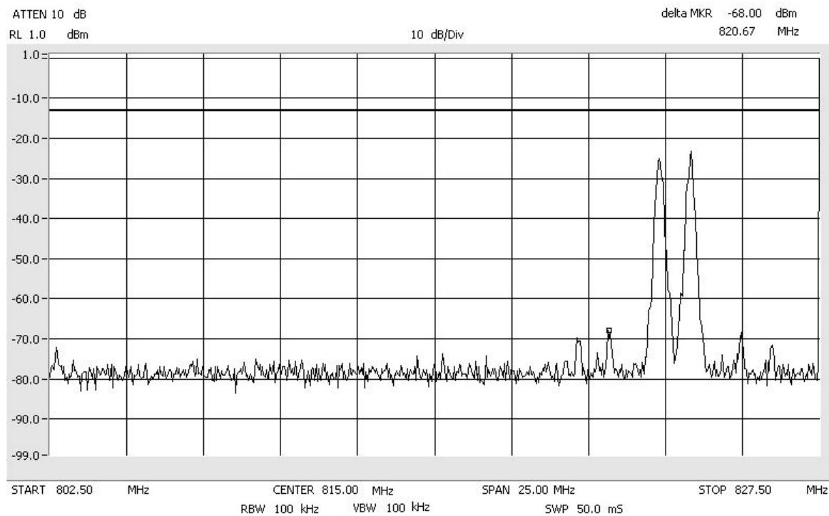
Intermodulation      iDEN\_High      SMR\_800\_MHz
