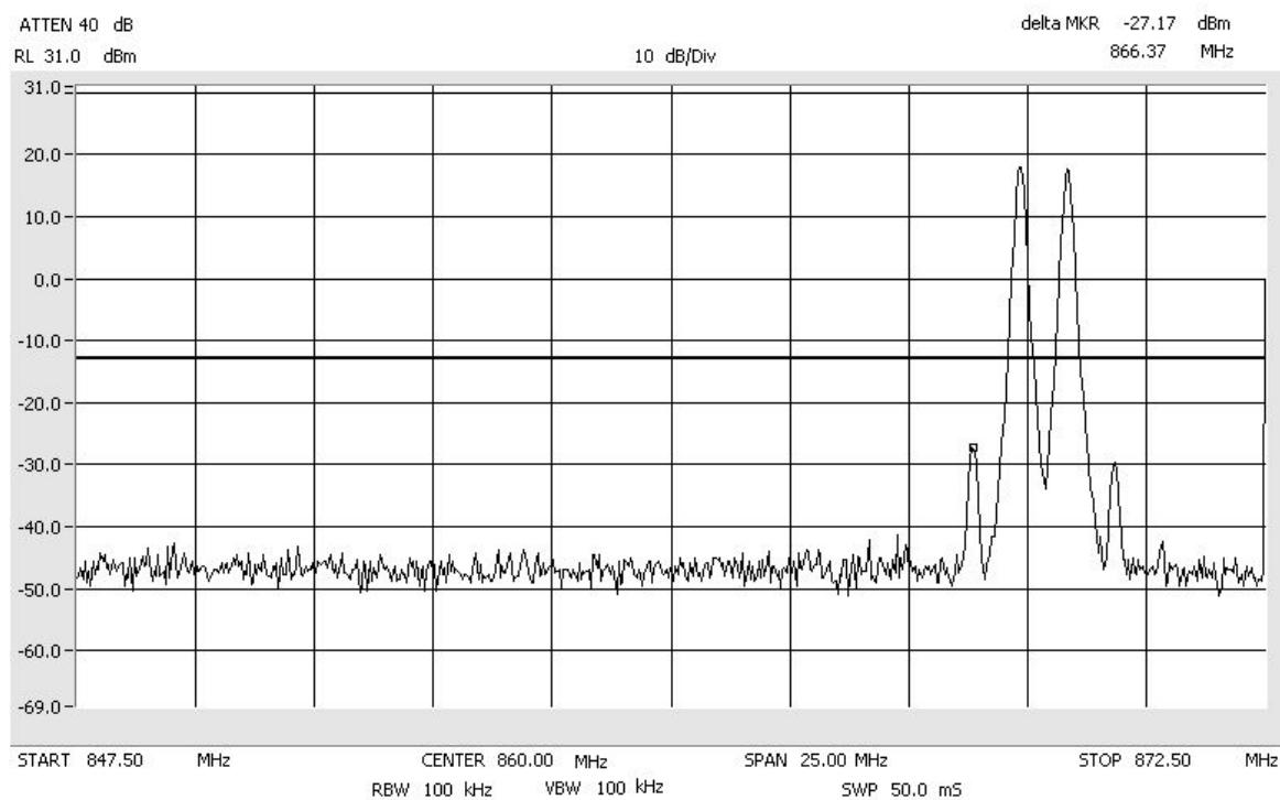
Intermodulation APCO25\_CQPSK\_High SMR\_800\_MHz
