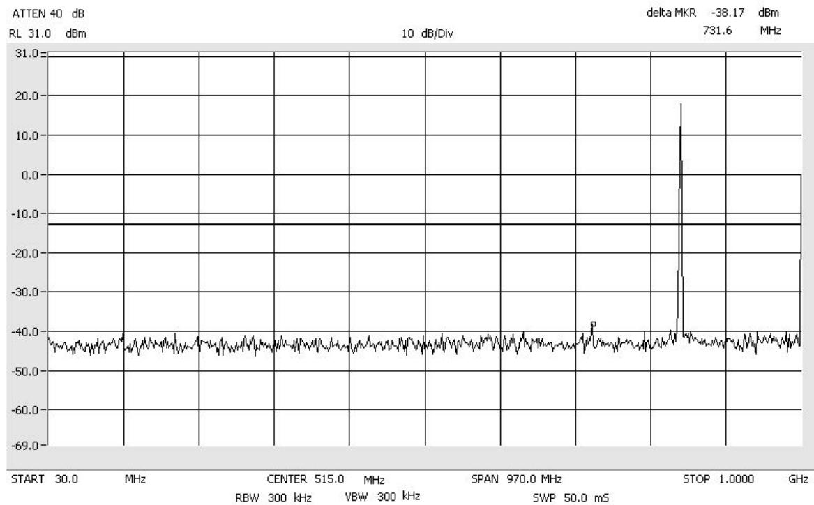
Intermodulation iDEN\_Low SMR\_800\_MHz
