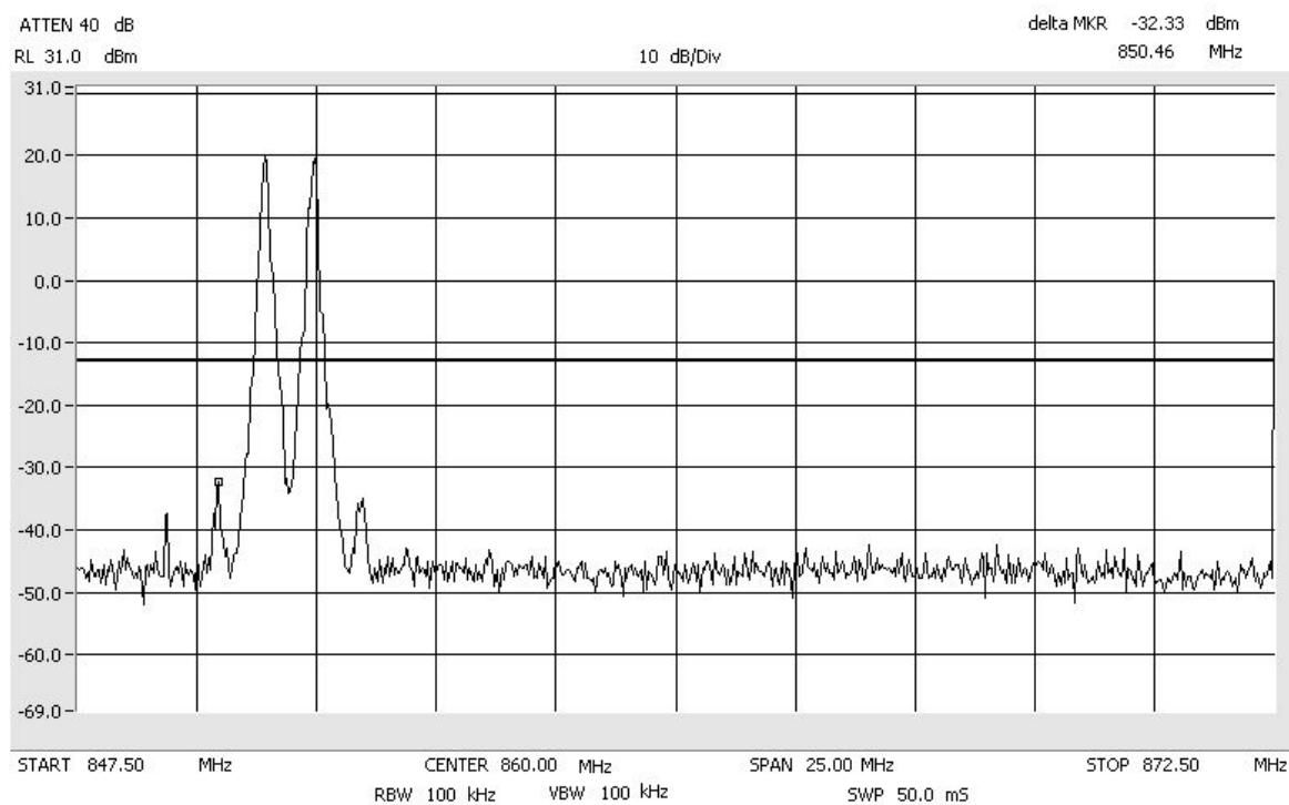
Intermodulation APCO25\_C4FM\_Low SMR\_800\_MHz
