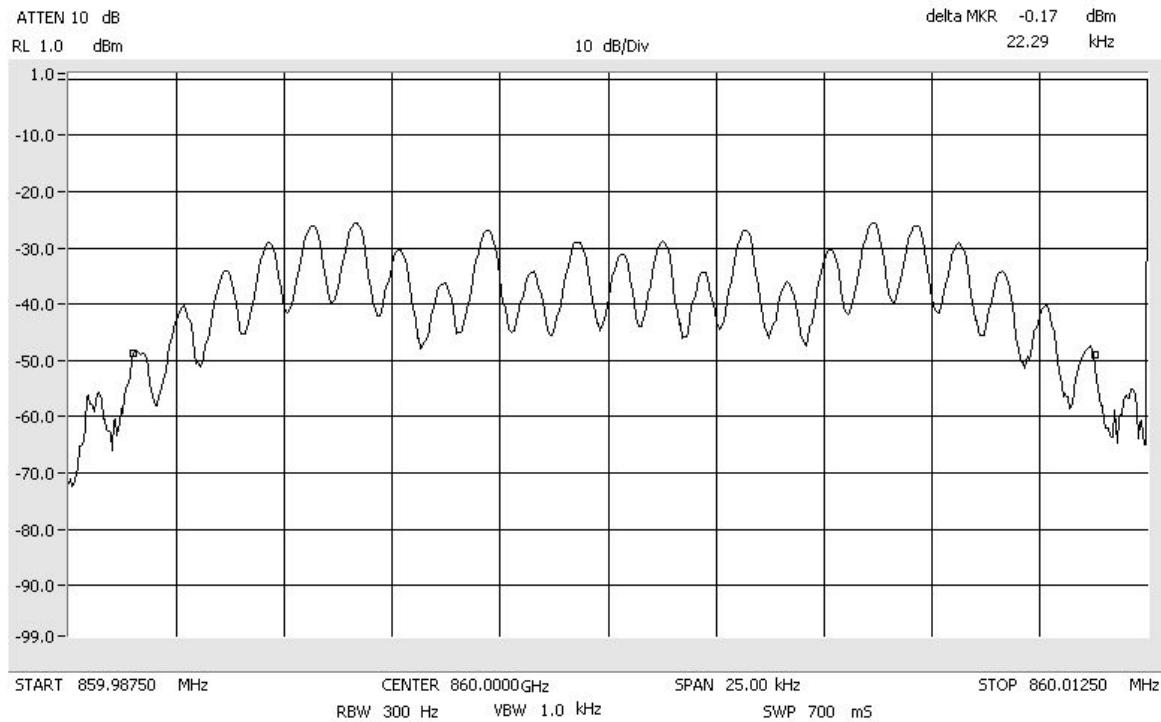
Occupied Bandwidth iDEN\_Signal\_In
