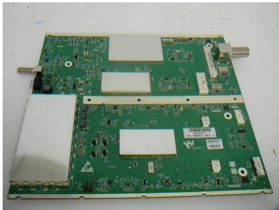
**13.7 EUT – PCB Board View (1) without Shielding**
