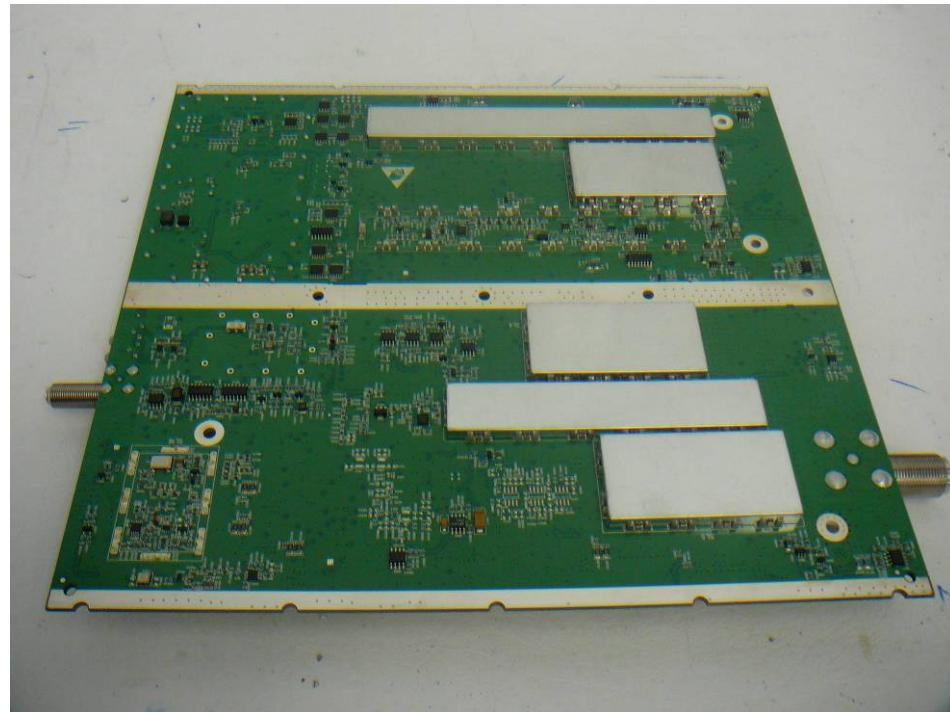
**13.9 EUT – PCB Board View (2) Without Shielding**
