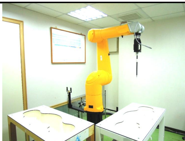
Fig-3.2 SPEAG DASY52 System
