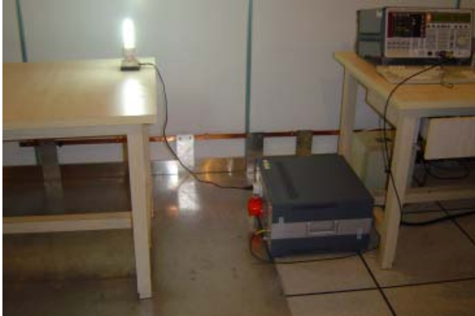
Conducted Emission Test Setup View for DEF-20W
