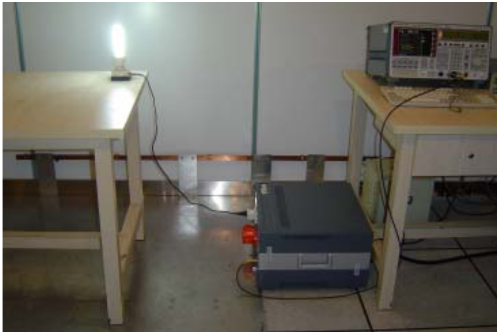
Conducted Emission Test Setup View for DEF-20W
