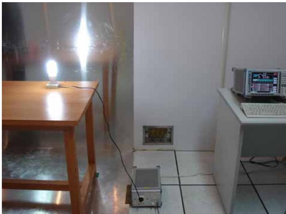
**Conducted Emission Test View For DEC3H Series 32W**
