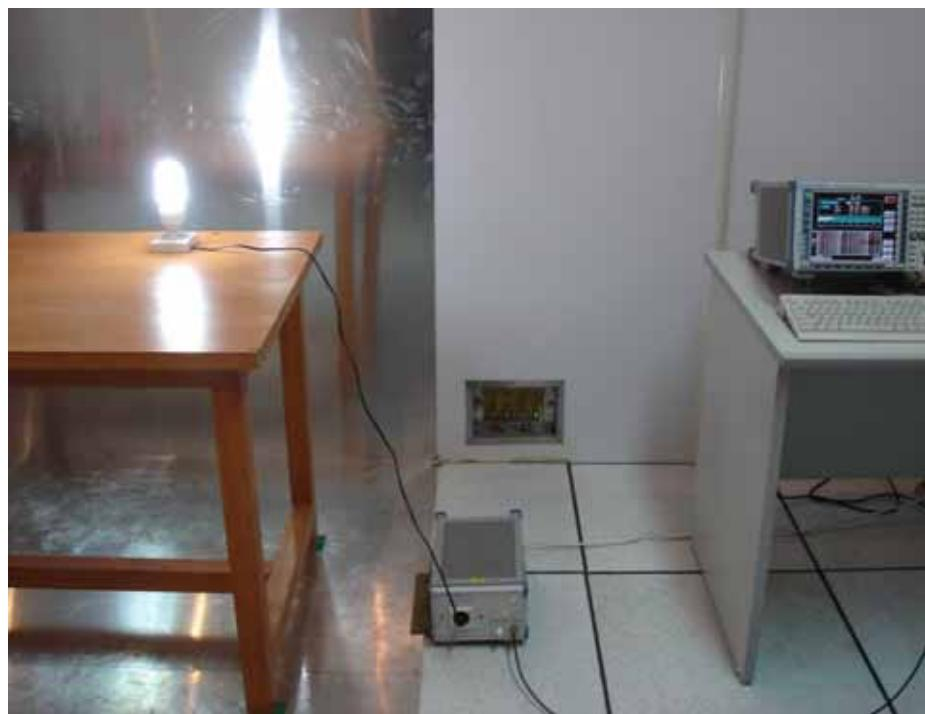
**Conducted Emission Test View For DEC3H Series 30W**
