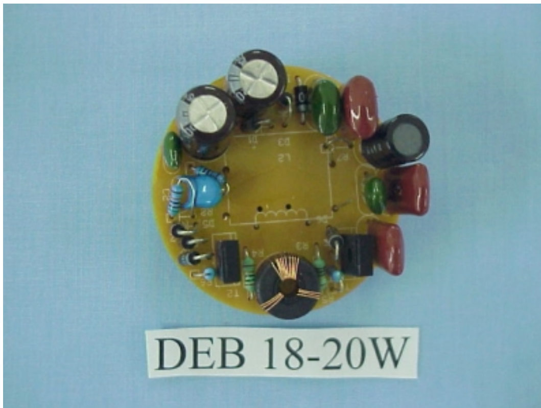
FIGURE 6 ELECTRONIC ENERGY SAVING LAMP (M/N: DEB/18~20W) MAIN BOARD (COMPONENT SIDE)
