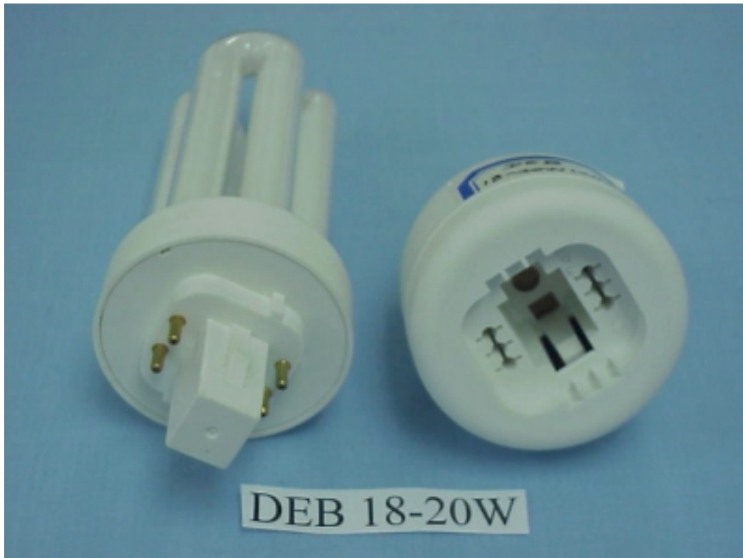
FIGURE 5 ELECTRONIC ENERGY SAVING LAMP (M/N: DEB/18~20W) LAMP TUBE AND LAMP HOLDER SEPARATED
