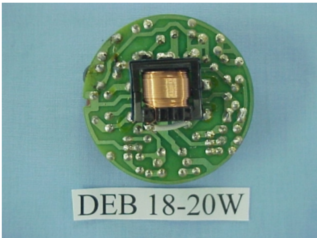
FIGURE 7 ELECTRONIC ENERGY SAVING LAMP (M/N: DEB/18~20W) MAIN BOARD (SOLDERED SIDE)
