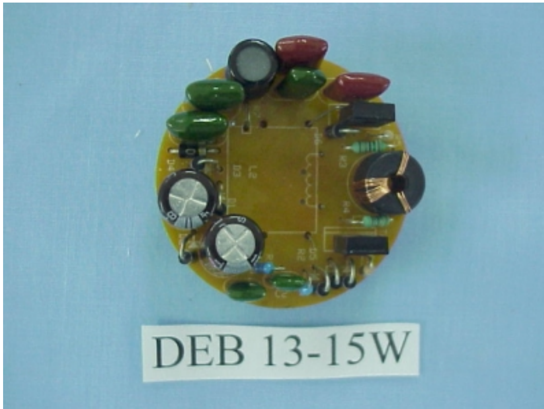
FIGURE 3 ELECTRONIC ENERGY SAVING LAMP (M/N: DEB/13~15W) MAIN BOARD (COMPONENT SIDE)
