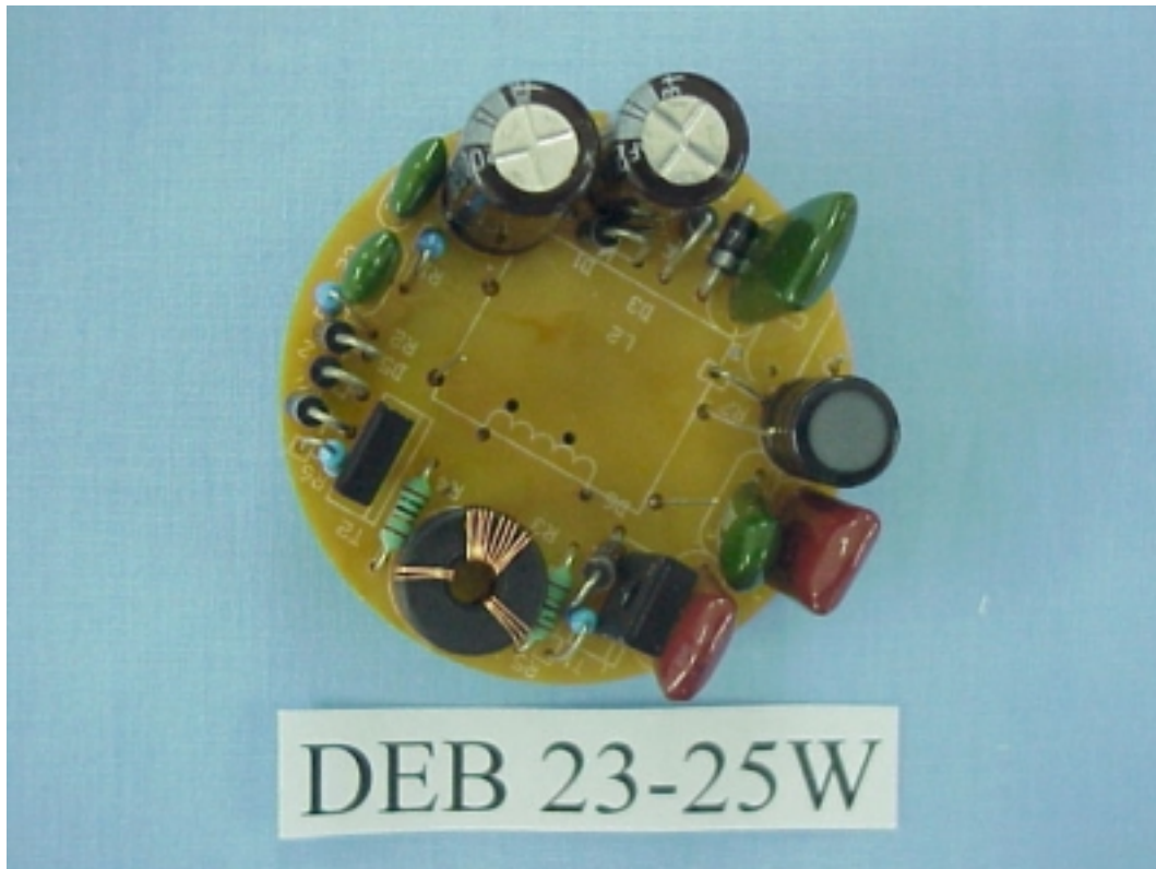
FIGURE 9 ELECTRONIC ENERGY SAVING LAMP (M/N: DEB/23~25W) MAIN BOARD (COMPONENT SIDE)
