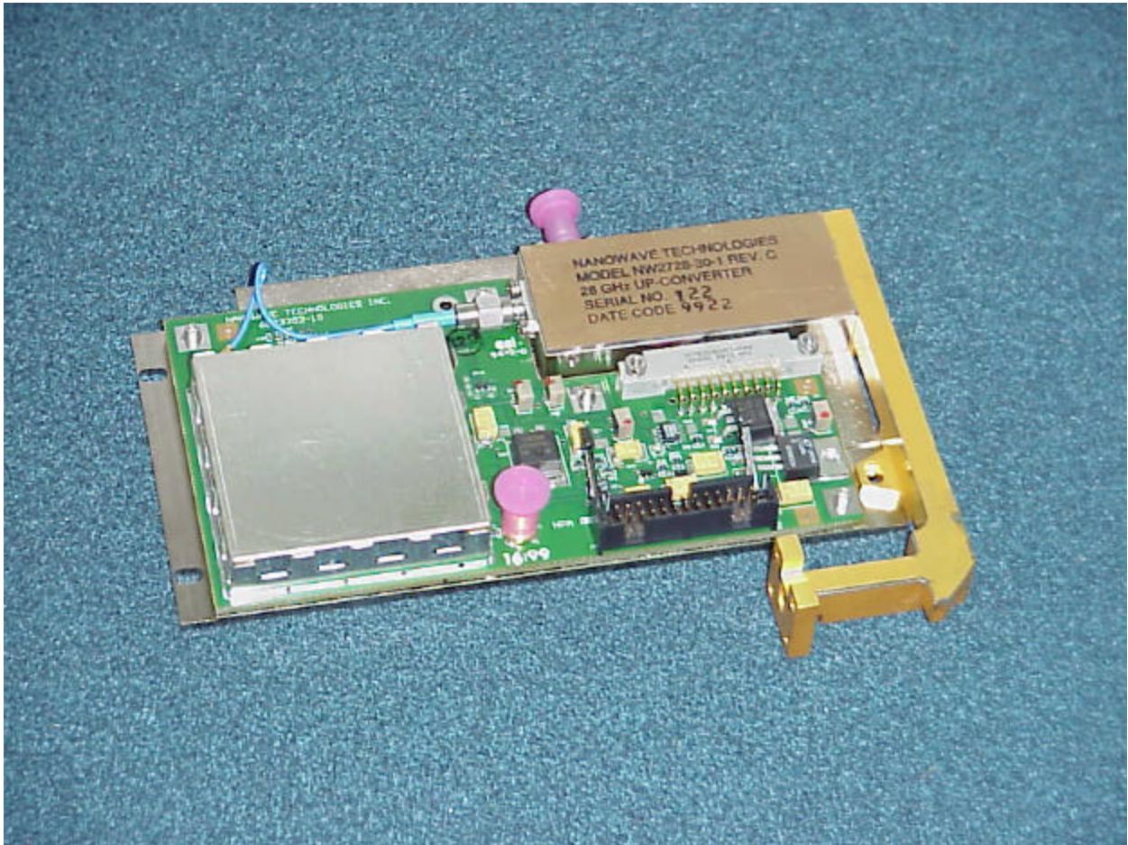
Figure 9-7 Node Transmitter High Power Amplifier
