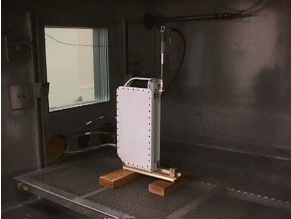
Figure 7-5 SpectraPoint High Gain Node Transmitter Setup for Frequency Stability Testing in the Temperature Chamber
