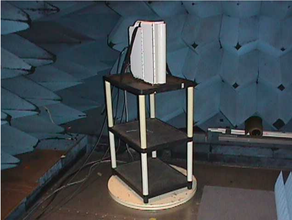
Figure 7-3 SpectraPoint High Gain Node Transmitter Setup for Radiated Spurious Emissions Testing
