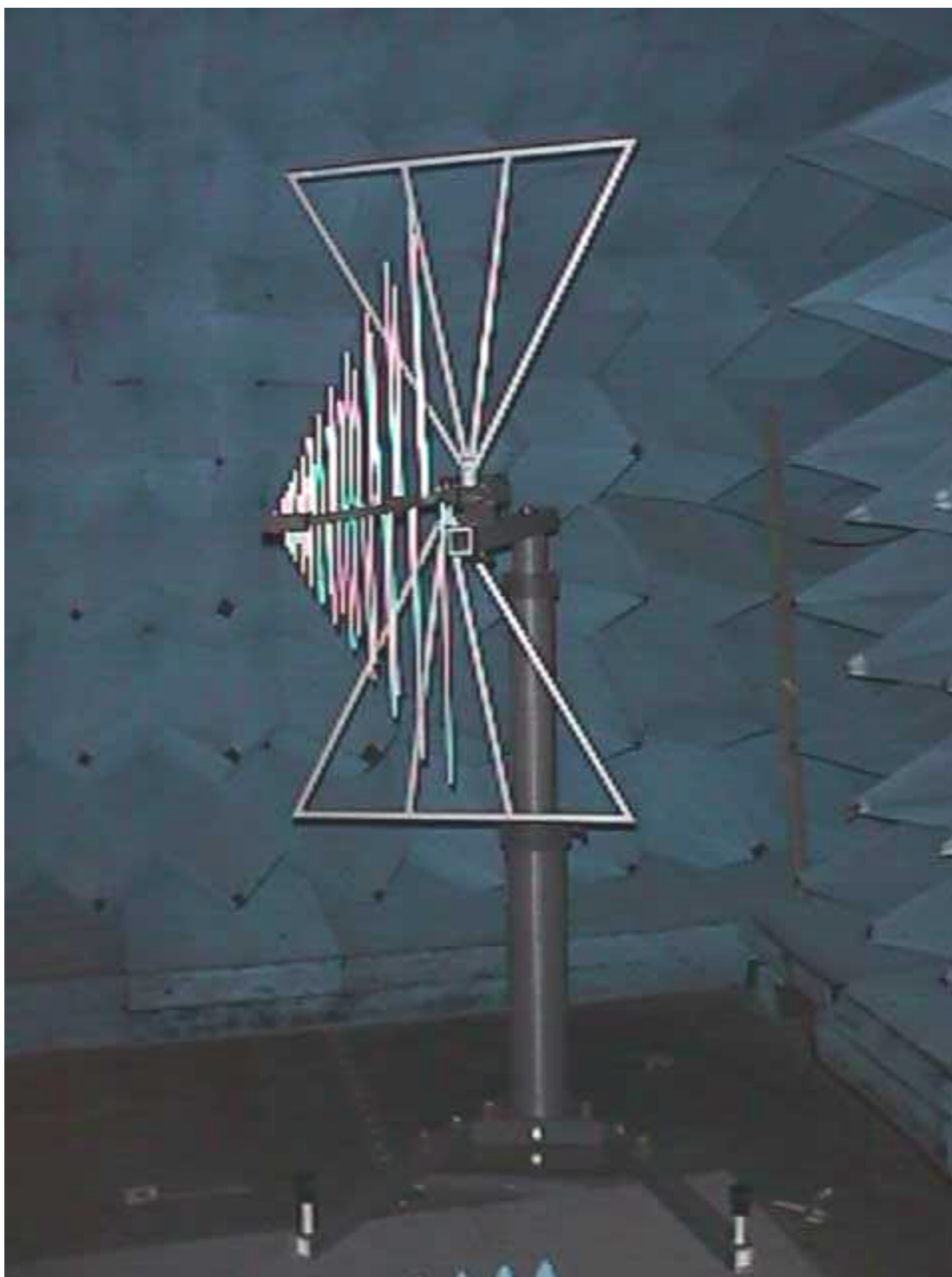
Figure 7-4 Setup of BiConiLog Antenna for Measurement of Radiated Spurious Emissions from the SpectraPoint High Gain Node Transmitter
