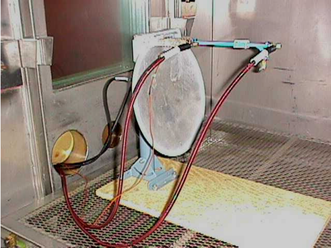
Figure E – 2 SpectraPoint CPE Roof Unit Transceiver Setup for Frequency Stability Testing in the Temperature Chamber
