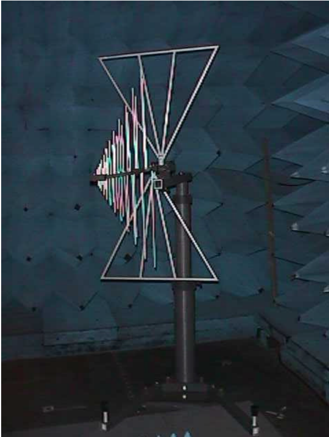
Figure B – 8 Setup of BiConiLog Antenna for Measurement of Radiated Spurious Emissions from the SpectraPoint CPE Roof Unit Transceiver
