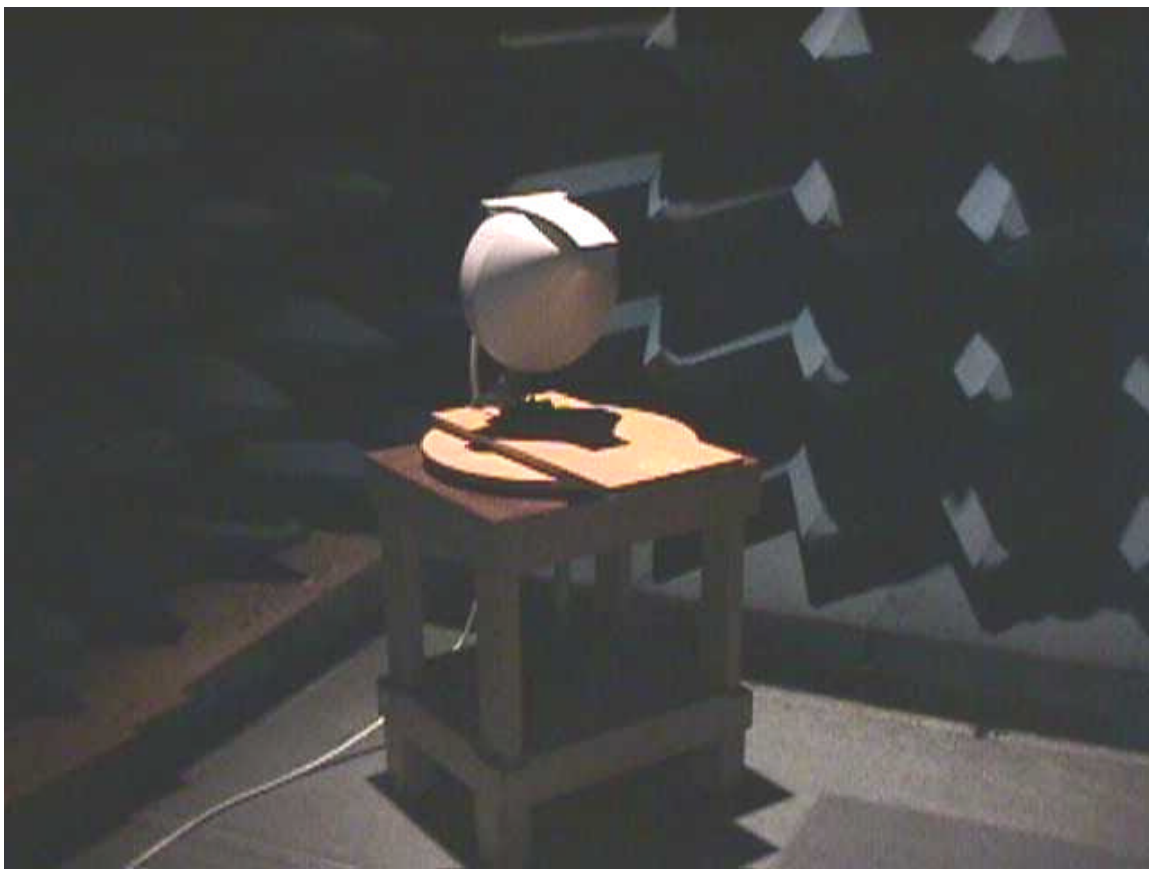
Figure B – 7 SpectraPoint CPE Roof Unit Transceiver Setup for Radiated Spurious Emissions Testing
