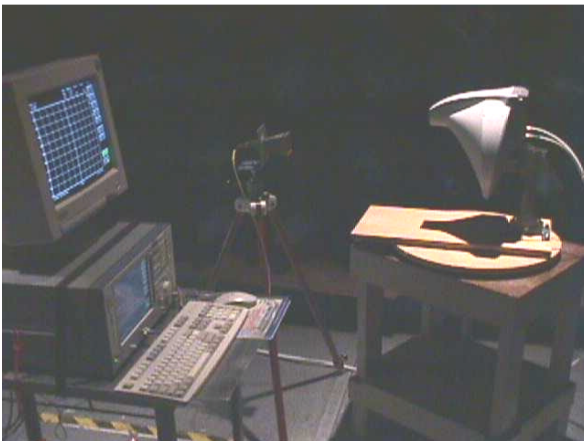
Figure A – 9 Test Setup for Antenna Radiated Emission Measurements on the SpectraPoint CPE Roof Unit Transceiver
