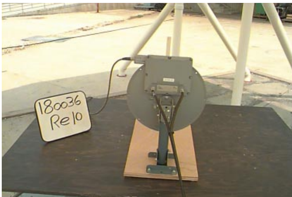
Configuration: Lower Frequency (Actual QPSK Signal) FIGURE D-5. WORST-CASE FIELD STRENGTH OF SPURIOUS RADIATED EMISSIONS ACTUAL QPSK SIGNAL (SCAN: 30 MHz – 1000 MHz) TEST SETUP
