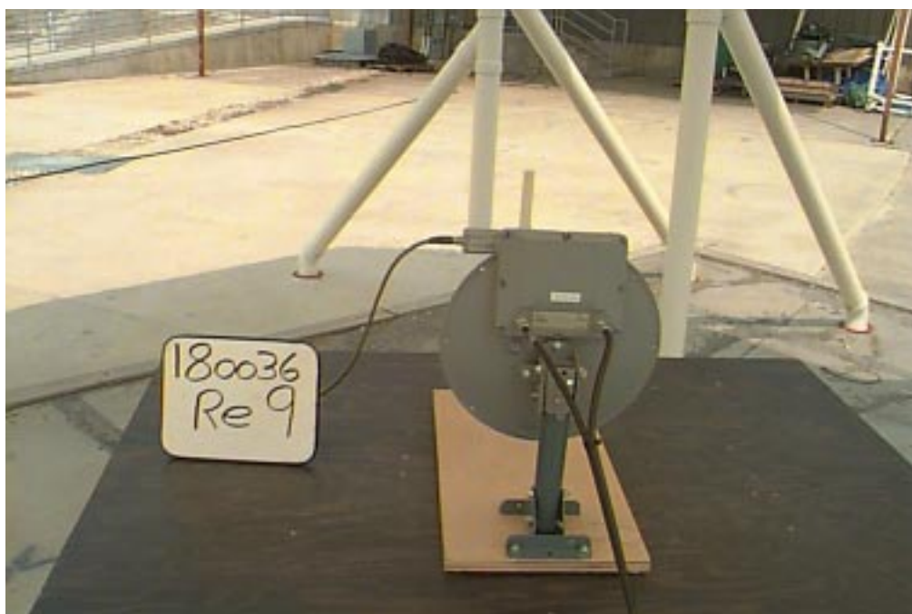
Configuration: Center Frequency (Actual QPSK Signal) FIGURE D-5. WORST-CASE FIELD STRENGTH OF SPURIOUS RADIATED EMISSIONS ACTUAL QPSK SIGNAL (SCAN: 30 MHz – 1000 MHz) TEST SETUP (Continued)
