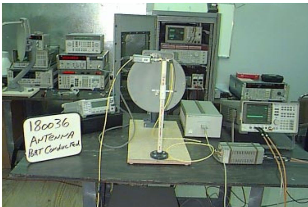
FIGURE D-4 SPURIOUS EMISSIONS AT ANTENNA TERMINALS TEST SETUP
