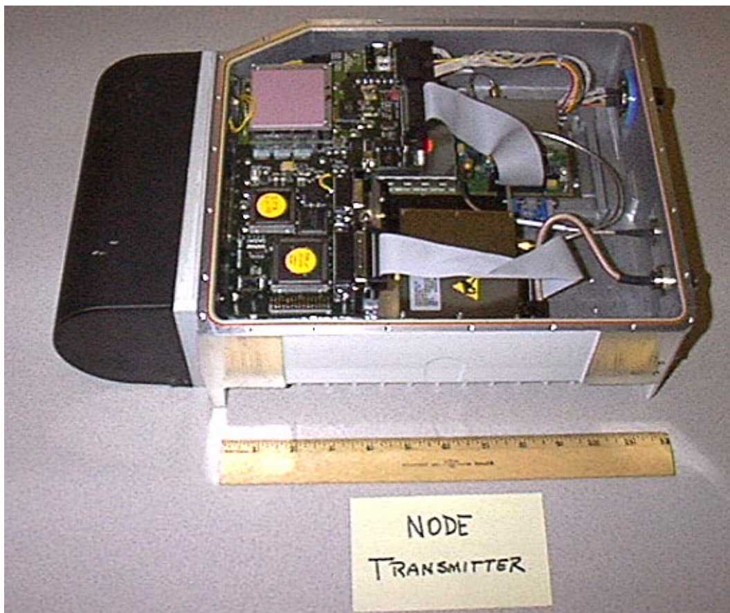
Figure 9-9 Transmitter in Redesigned Chassis with Chassis Cover Removed
