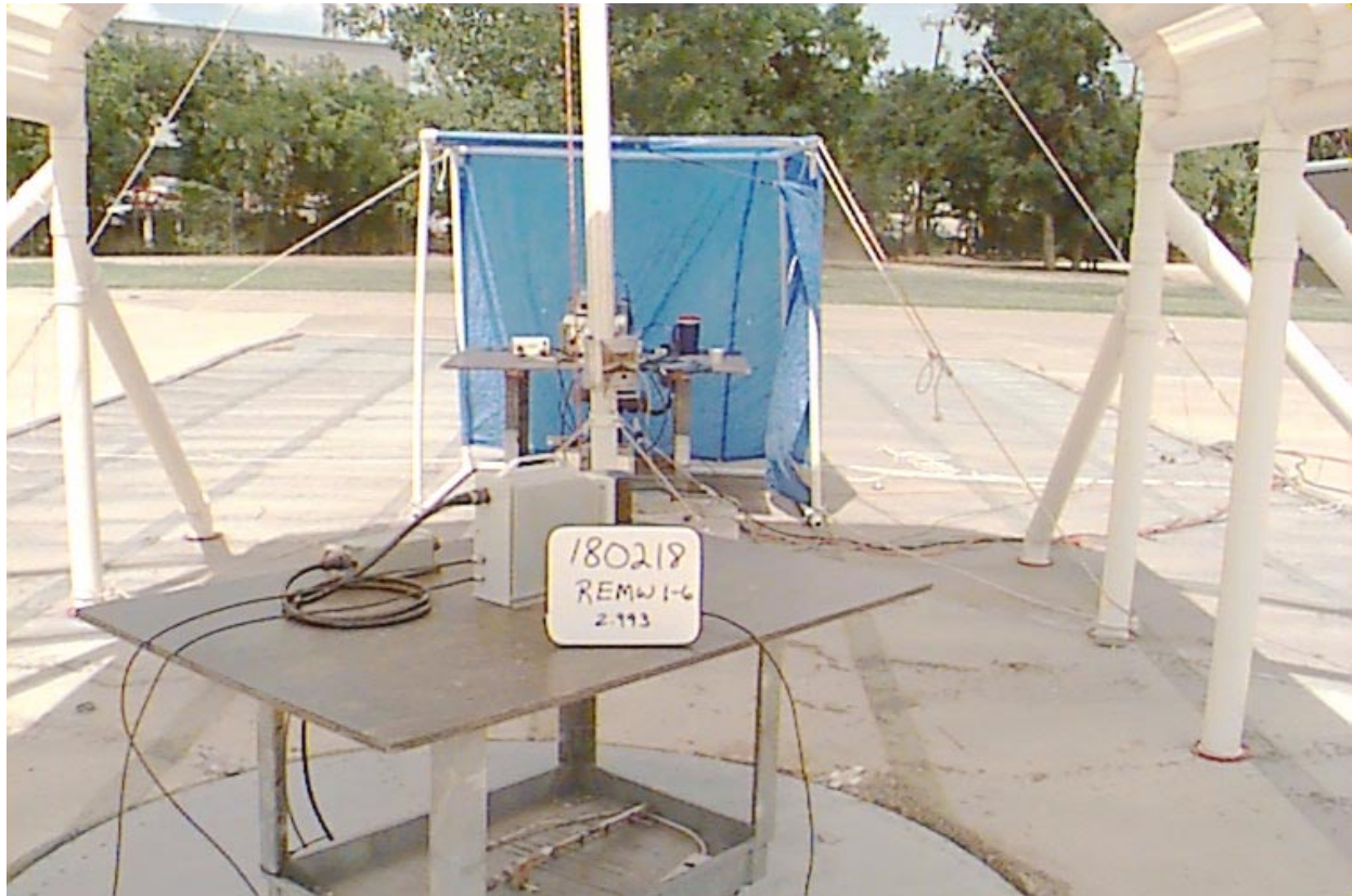
Figure 7-4 Test Setup for Spurious Radiated Emission Measurements
