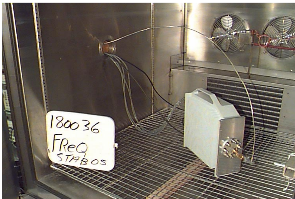
Figure 7-5 Test Setup for Temperature Stability Measurements
