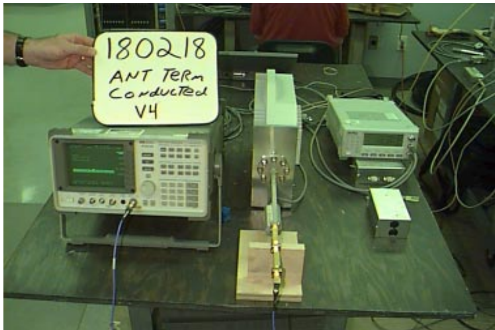
FIGURE D-3. ANTENNA TEMINAL CONDUCTED EMISSIONS TEST SETUP (Continued)
