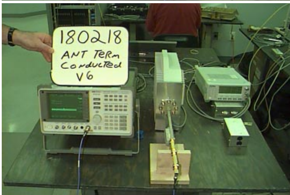
FIGURE D-3. ANTENNA TERMINAL CONDUCTED EMISSIONS TEST SETUP (Conducted)
