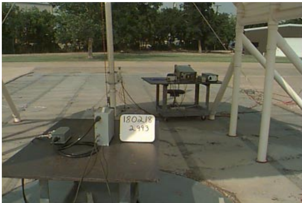
FIGURE D-5. WORST-CASE SPURIOUS EMISSIONS (MICROWAVE FIELD STRENGTH) TEST SETUP
