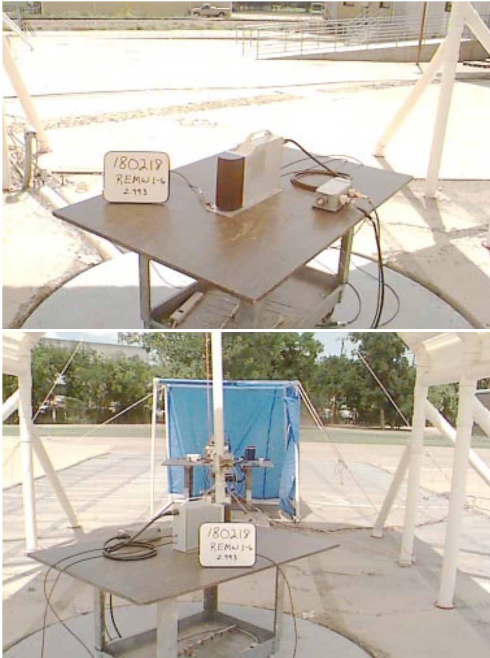
FIGURE D-5. WORST-CASE SPURIOUS EMISSIONS (MICROWAVE FIELD STRENGTH) TEST SETUP
