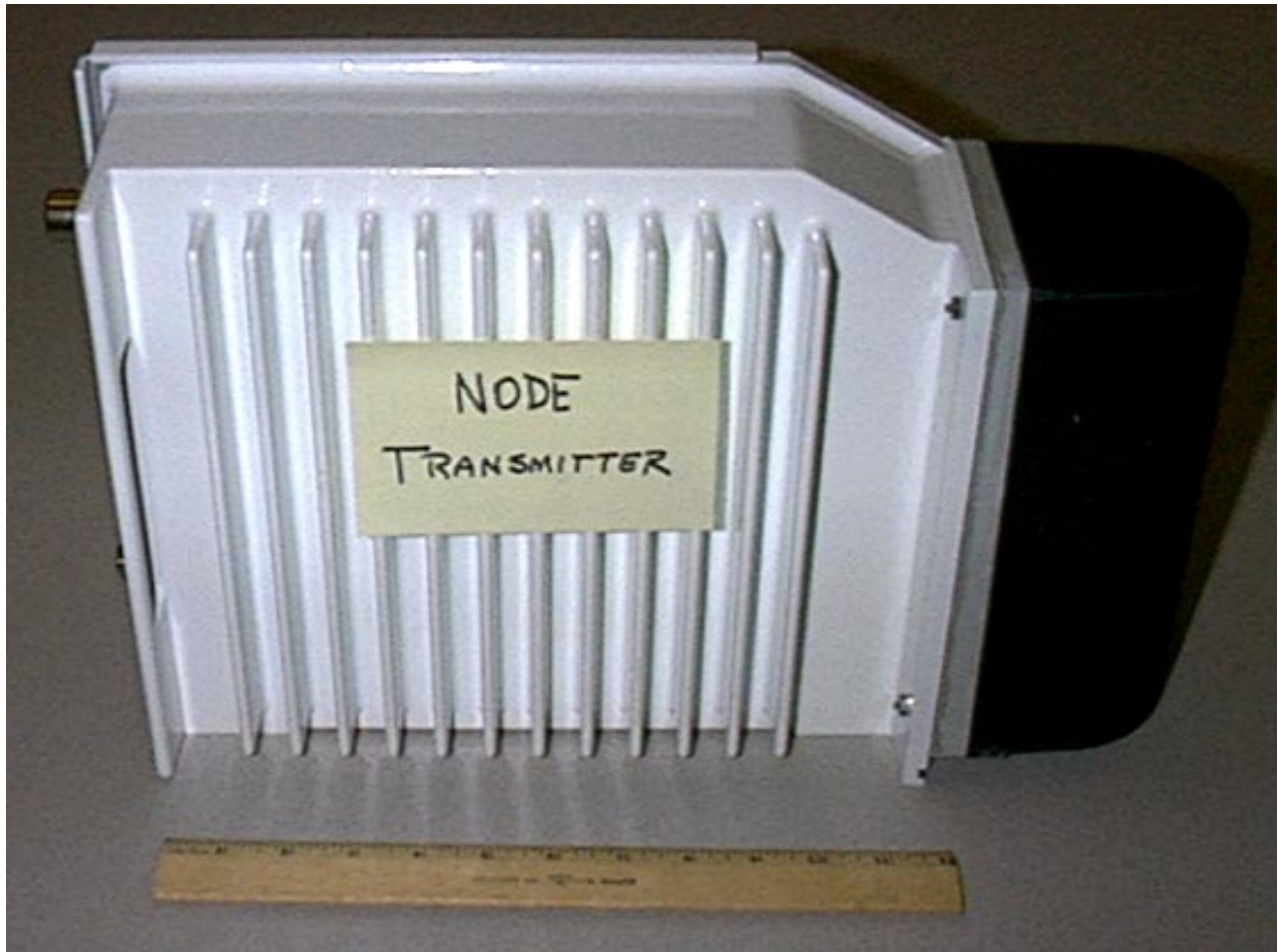
Figure 3-5 Transmitter Mounted in Redesigned Chassis (Heat Sink Side)
