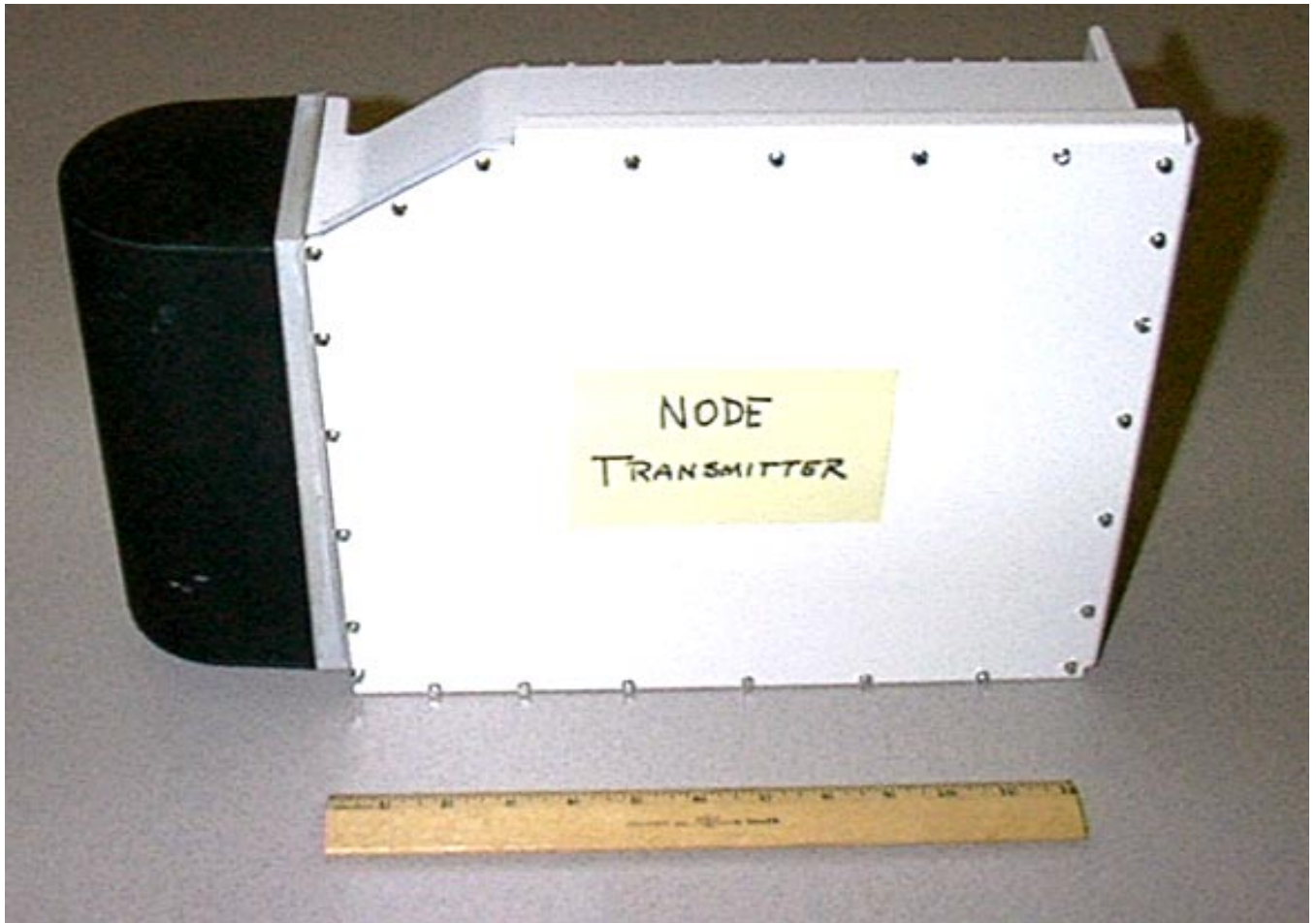
Figure 3-4 Transmitter Mounted in Redesigned Chassis (Cover Side)
