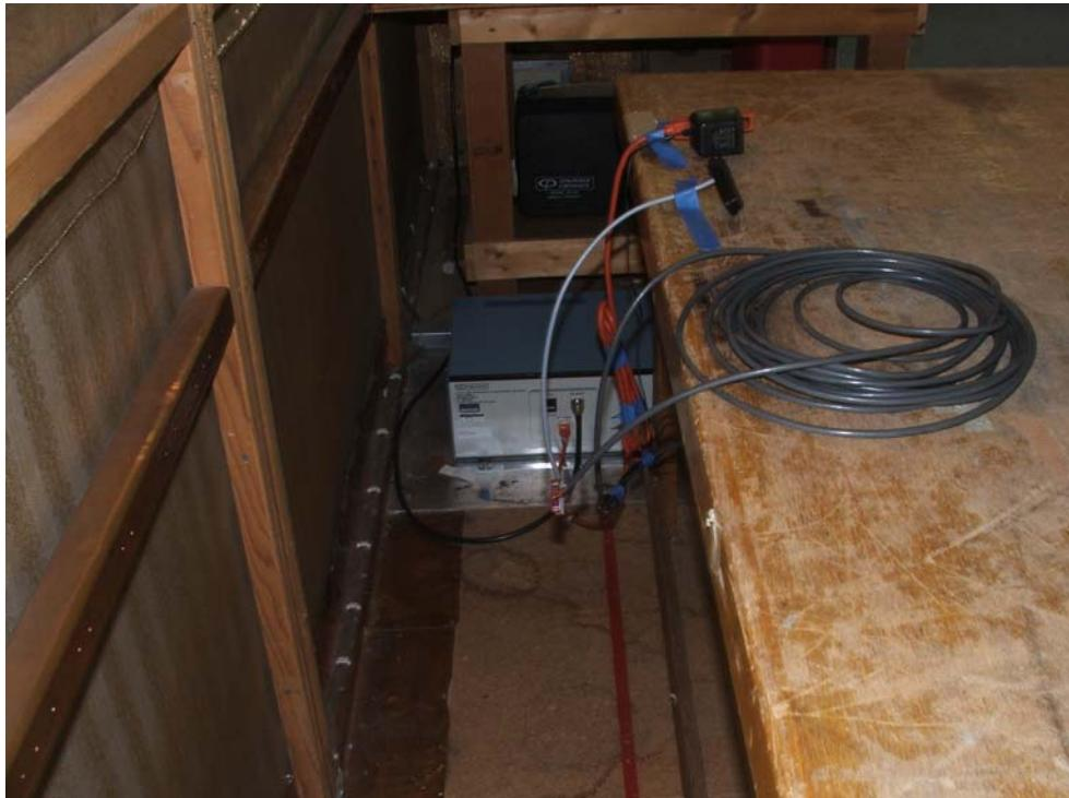
**REAR VIEW****SECURA KEY****ACCESS CONTROL SYSTEM****MODEL: AM-DPR (RKDT-W) (AM-DPR/RKDT-W)****FCC PART 15 SUBPART C - CONDUCTED EMISSIONS – 3-16-11****PHOTOGRAPH SHOWING THE EUT CONFIGURATION
