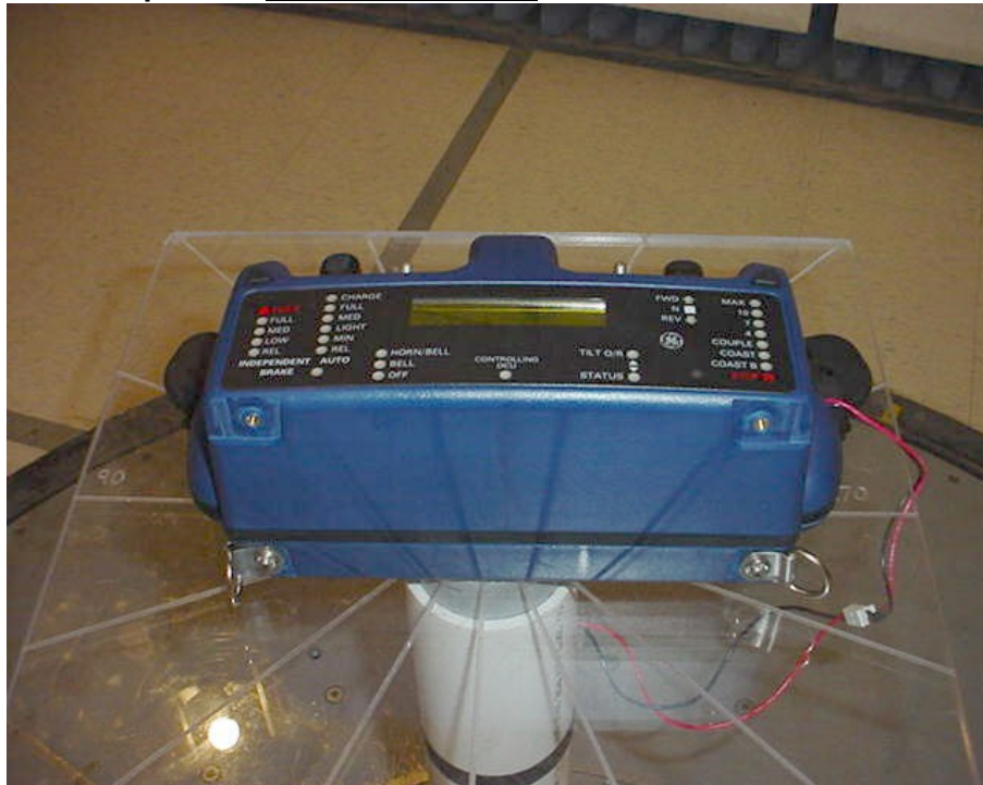
Setup for the Radiated Emissions Test , Horizontal Orientation
