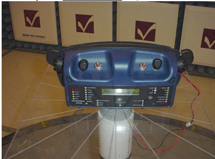
Setup for the Radiated Emissions Test , Vertical Orientation
