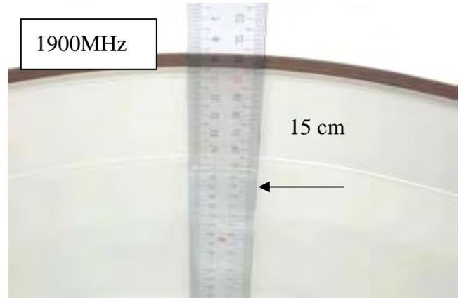
Fig.2.5 Photograph of the Tissue Simulant Fluid liquid depth 15cm for Flat (Body)
