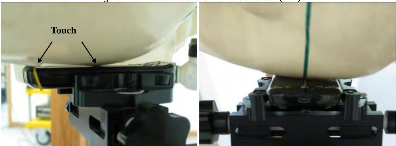
Fig.11 Right Head Section / Cheek-Touch Position
