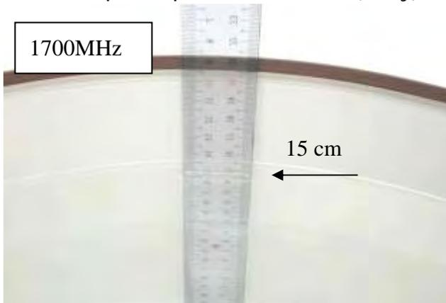
Fig.2.6 Photograph of the Tissue Simulant Fluid liquid depth 15cm for Flat (Body)
