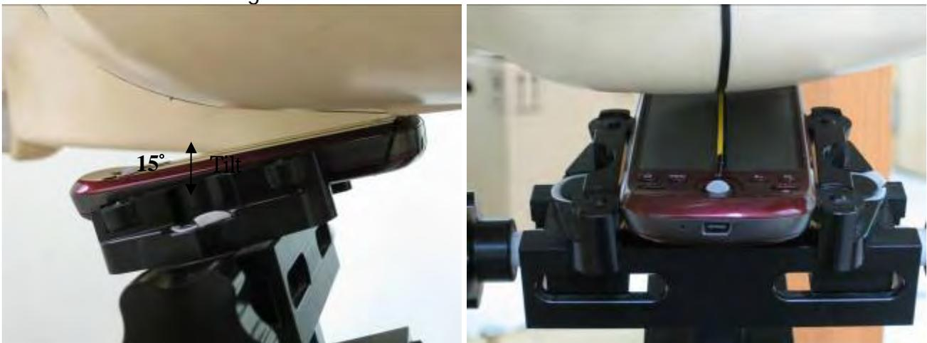
Fig.10 Left Head Section / Ear-Tilt Position(15°)
